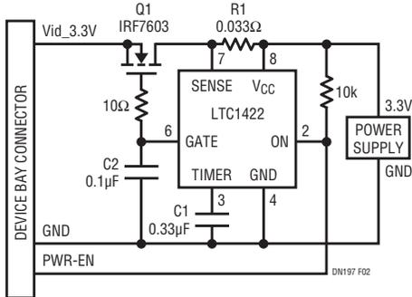
**Figure 2. Vid\_3.3V Supply Solution for DB32, DB20 and DB13 Form Factors**
