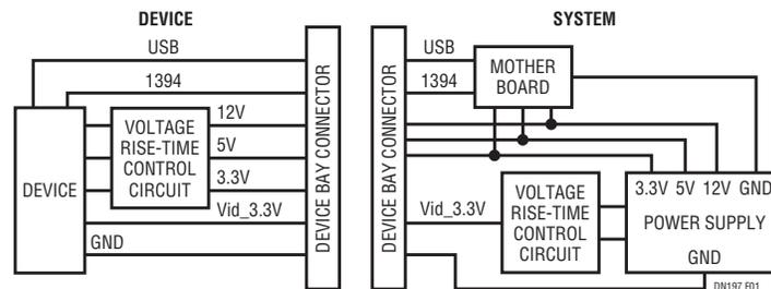
**Figure 1. Block Diagram for the Device Bay**
