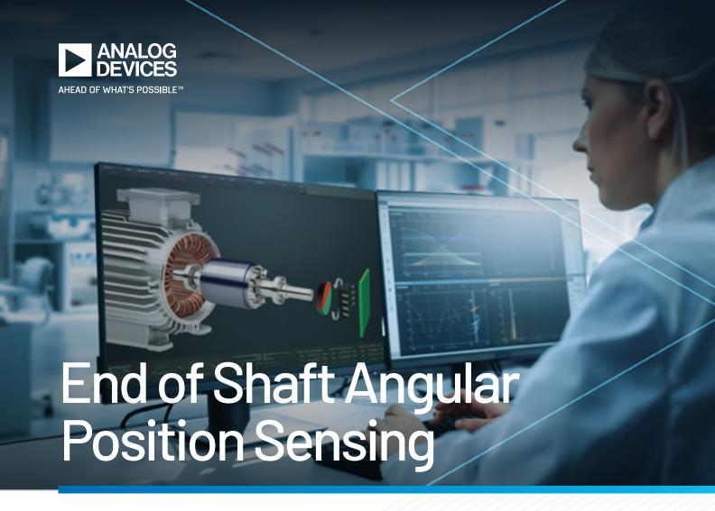
End of shaft position sensing is a type of contactless position sensing that makes use of a magnet attached to the end of a rotating shaft and an AMR sensor to measure the change in magnetic field direction to infer the position of the shaft relative to the sensor.
