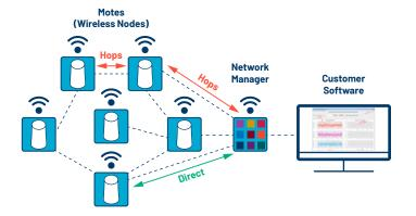
The Voyager kit supports ADI SmartMesh® mote hopping. This is where a mote, which is out of range of the network manager, can hop through an in-range mote. The multiple hops network ensures that out-of-range motes can stream data to the network manager, which extends the reach and the scale of the solution deployment.
