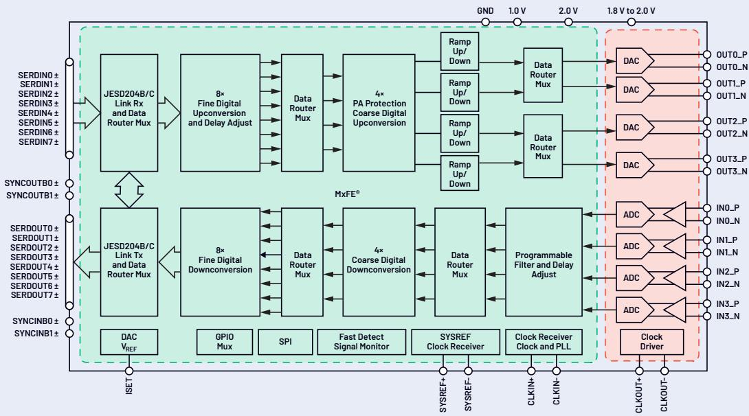
**The green block** highlights the on-chip DSP including a programmable FIR filter and coarse/fine decimation filters on the receive path and coarse/fine interpolation filters on the transmit path.
