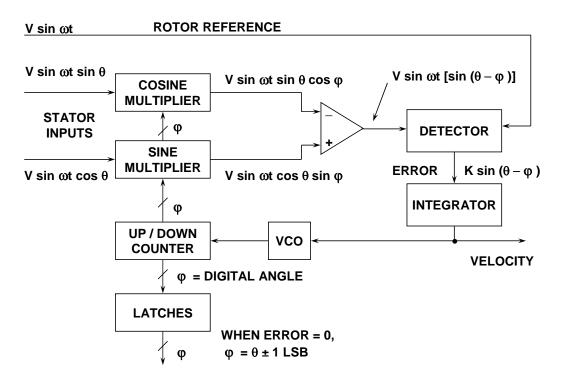
Figure 2: Resolver-to-Digital Converter (RDC)
