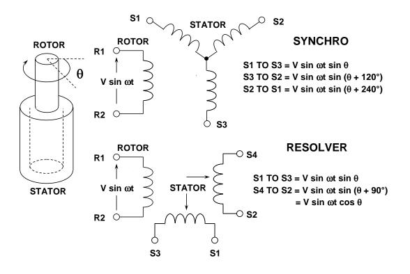
Figure 1: Synchros and Resolvers
