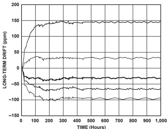
Figure 1. Typical Long-Term Drift Over 1,000 Hours
