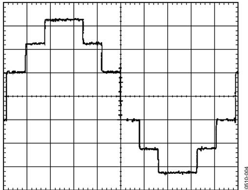
Figure 4. Nonideal Input AC Source 1 Waveform
