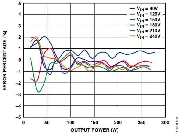
Figure 3. Measured Power Error with Ideal Input AC Source
