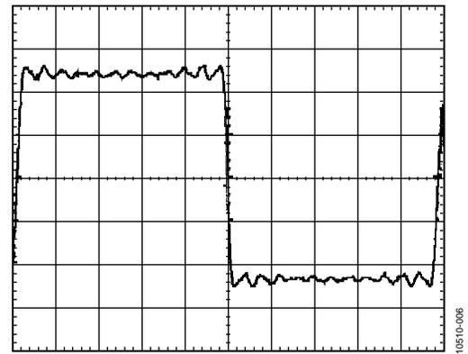
Figure 6. Nonideal Input AC Source 2 Waveform
