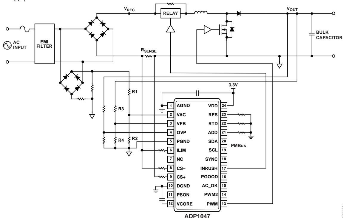
Figure 1. AC Power Metering Circuit Configuration
