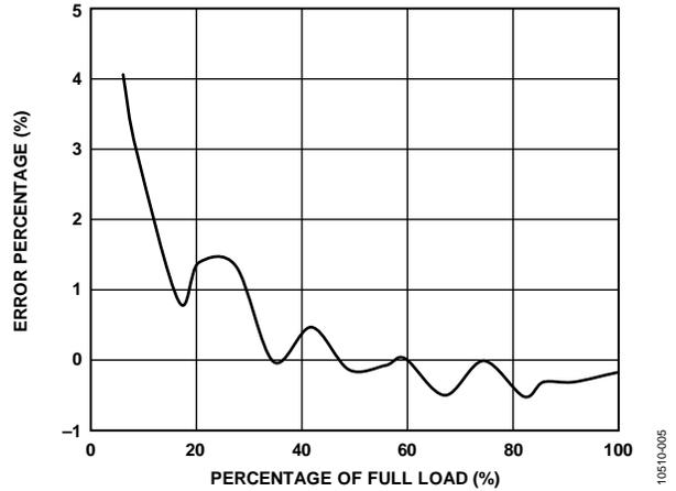
Figure 5. Measured Power Error with Nonideal Input AC Source 1
