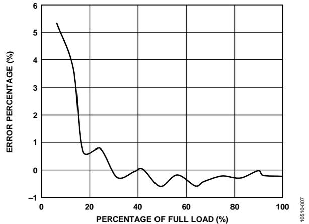
Figure 7. Measured Power Error with Nonideal Input AC Source 2
