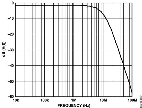
Figure 7. Baseband Filter Gain Response in Decibels
