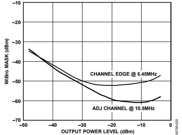
Figure 25. Transmitter Spectral Quality According to WiBro Mask (64 QAM WiMAX OFDM, 10 MHz BW) Function of Output Power or V\_GAIN Voltage
