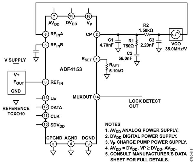
Figure 13. PLL Loop Schematic
