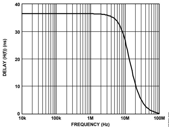
Figure 8. Baseband Filter Group Delay Response in Seconds
