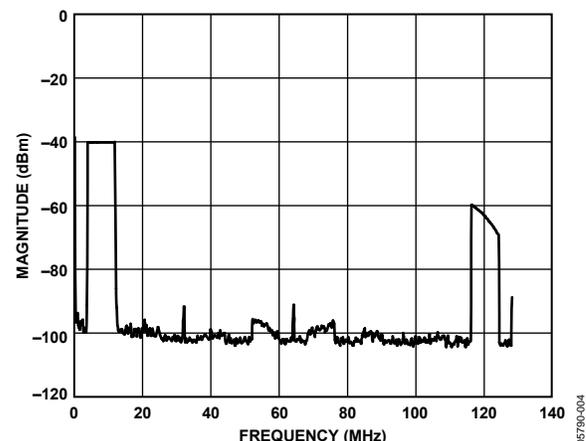
Figure 4. AD9860/AD9862 Tx DAC Generating an OFDM Signal with 4× Interpolation ( $f_{\text{SAMPLE}} = 32$  MSPS, 4× Interpolation)
