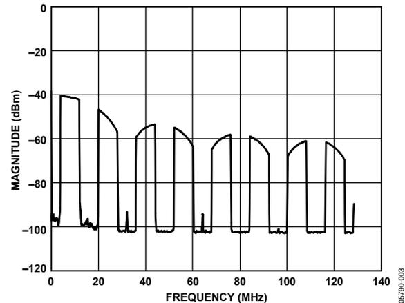
Figure 3. AD9860/AD9862 Tx DAC Generating an OFDM Signal with 1× Interpolation ( $f_{\text{SAMPLE}} = 32$  MSPS, 1× Interpolation)
