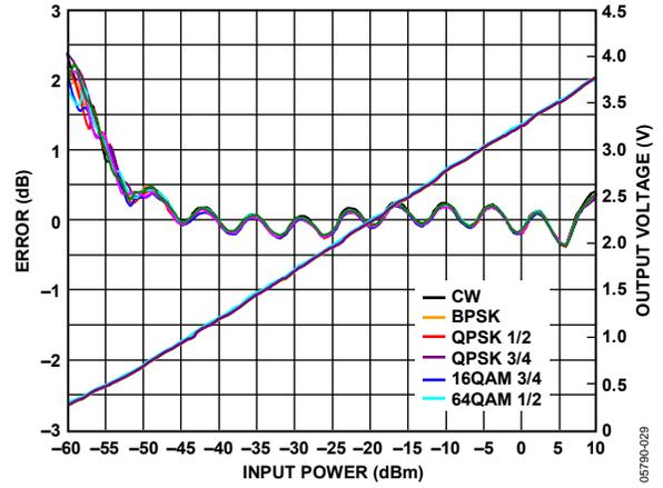
Figure 29. RMS Power Detector Response and Detection Error vs. Tx Signal Chain Output Power Level for QPSK, 16 QAM, 64 QAM OFDM Modulations
