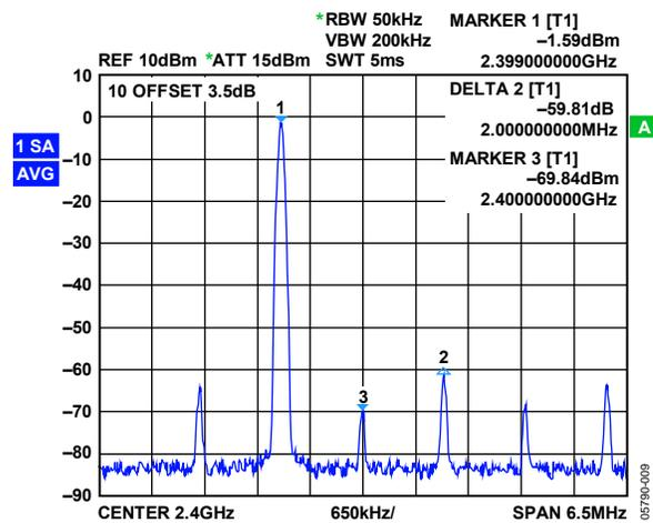
Figure 9. Single Sideband Spectrum at 2.4 GHz, After DC/Gain Calibration (DAC+IQ Modulator Output)
