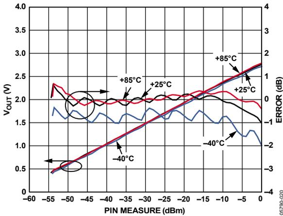
Figure 20. Output Voltage and Temperature Drift of the AD8362 at 2.35 GHz with External Temperature Compensation
