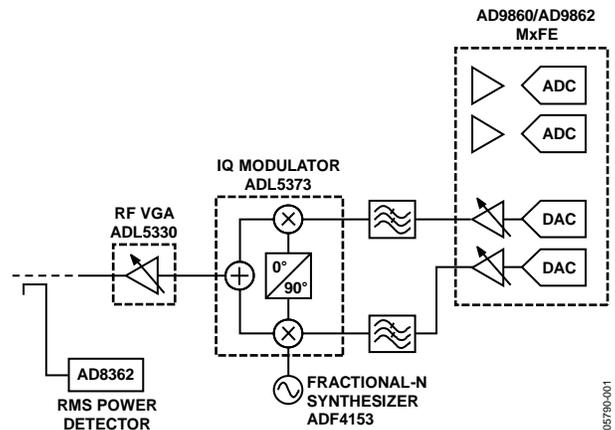
Figure 1. Direct Conversion Transmitter
