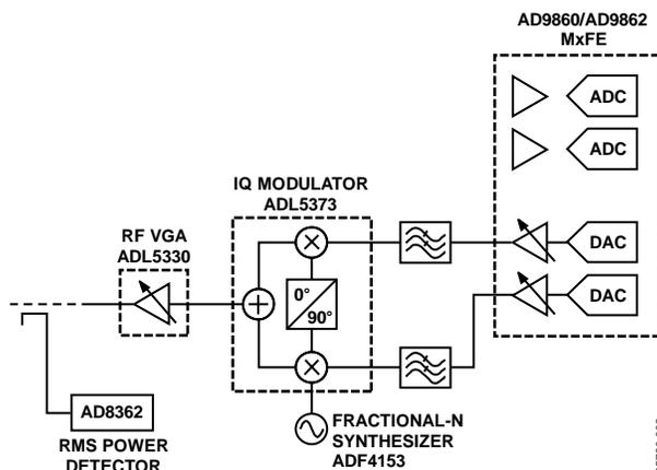
Figure 2. Direct Conversion Tx Chain
