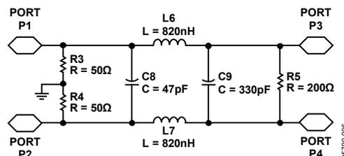
Figure 6. Baseband Filter Schematic Including Source Resistor and Termination Resistor
