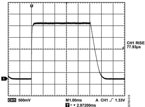
Figure 18. Power Detector Time Response to a WiMAX Downlink Burst (T<sub>SYMB</sub> = 25.6 μs), CLPF = 47 nF
