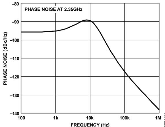
Figure 14. Closed-Loop Phase Noise Simulation at 2.35 GHz
