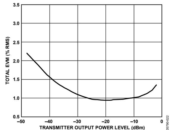
Figure 22. Signal Chain Total EVM as a Function of the Tx VGA Gain
