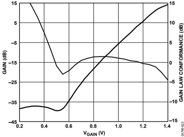
Figure 23. Power Gain Range for -10 dBm Out of the IQ Modulator, and Gain Law Conformance vs. V\_GAIN at 2350 MHz
