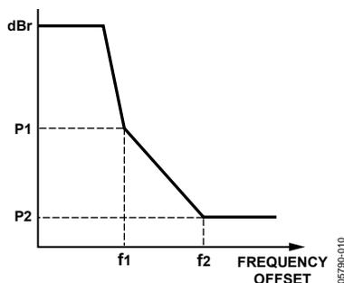
Figure 10. BTS WiBro Spectral Mask (RBW = 100 kHz)
