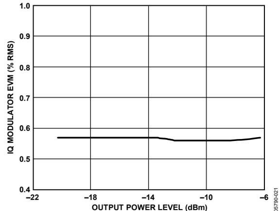
Figure 21. IQ Modulator EVM in %rms vs. Output Power, 64 QAM OFDM
