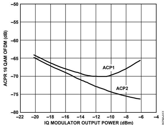
Figure 12. Modulator Output ACPR with 16 QAM OFDM Modulation, Function of I and Q Input Voltage (or IQ Modulator Output Power), at 2400 MHz
