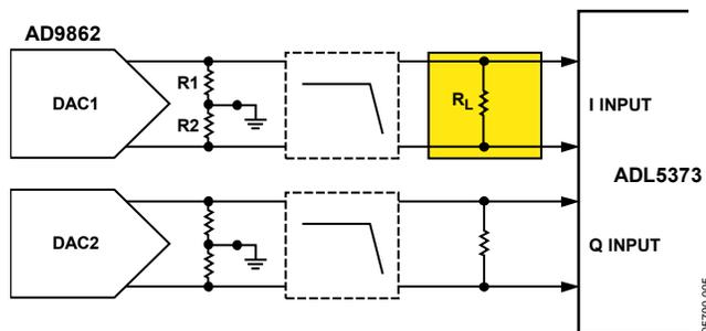
Figure 5. DAC to IQ Modulator Interface
