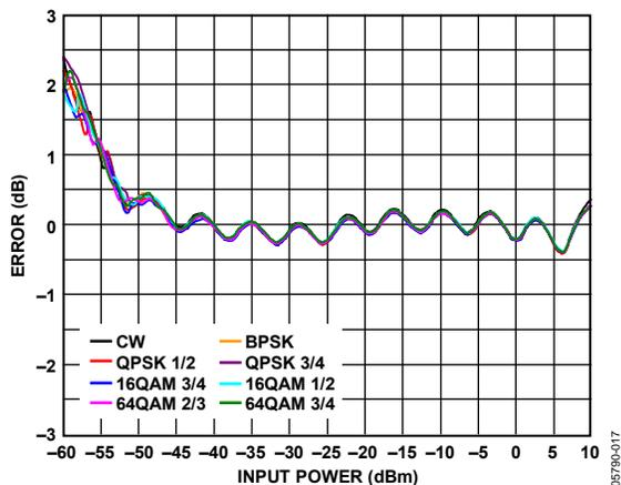
Figure 17. RMS Power Detector Detection Range and Accuracy for CLPF = 1 μF
