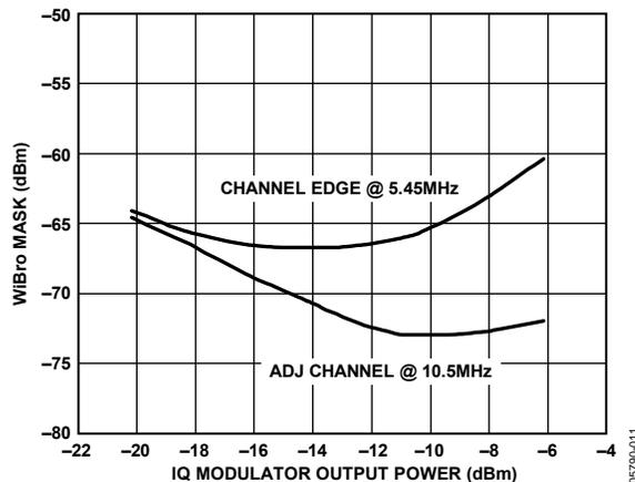
Figure 11. Modulator Performance According to WiBro Mask, with 16 QAM OFDM Modulation, Function of I and Q Input Voltage (or IQ Modulator Output Power), at 2400 MHz
