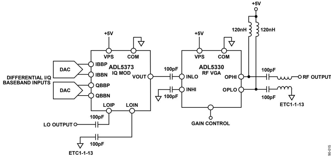
Figure 15. IQ Modulator and RF VGA Interfaces
