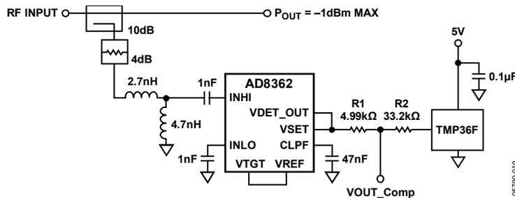
Figure 19. Power Detection and Temperature Compensation of the AD8362 at 2.35 GHz
