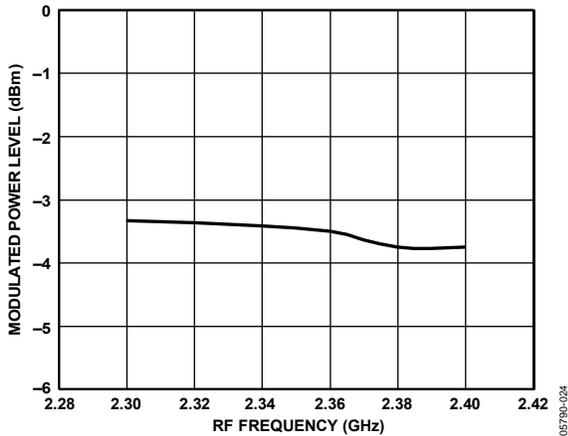
Figure 24. Modulated Power Level vs. RF Frequency, with a Modulated OFDM Signal
