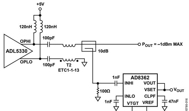
Figure 16. Power Detection Using the AD8362
