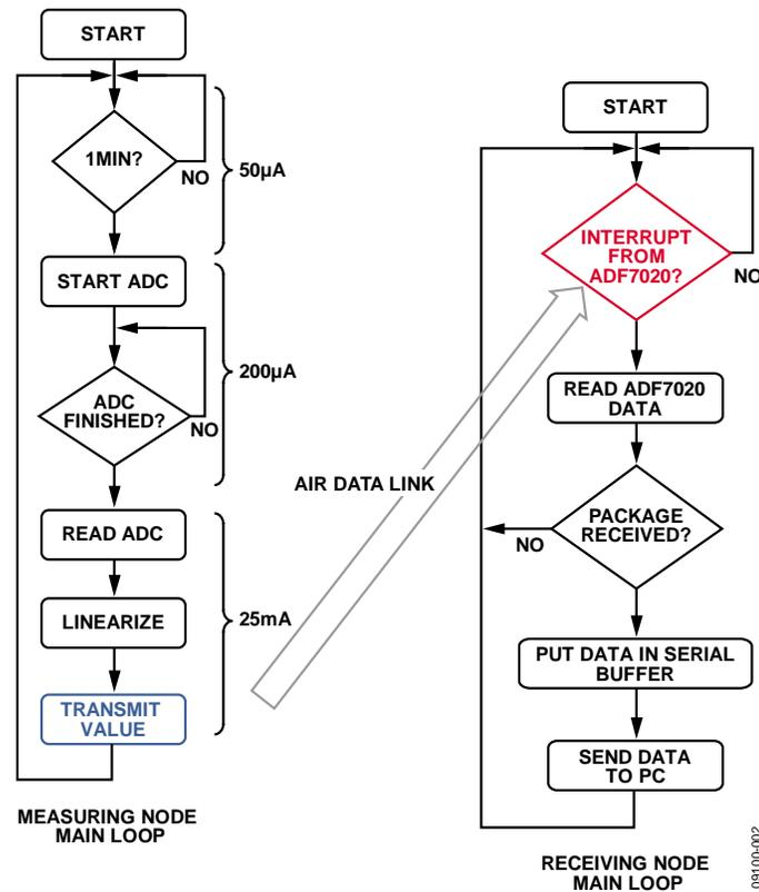
Figure 2. Measuring and Receiving Node Main Loop Flowcharts
