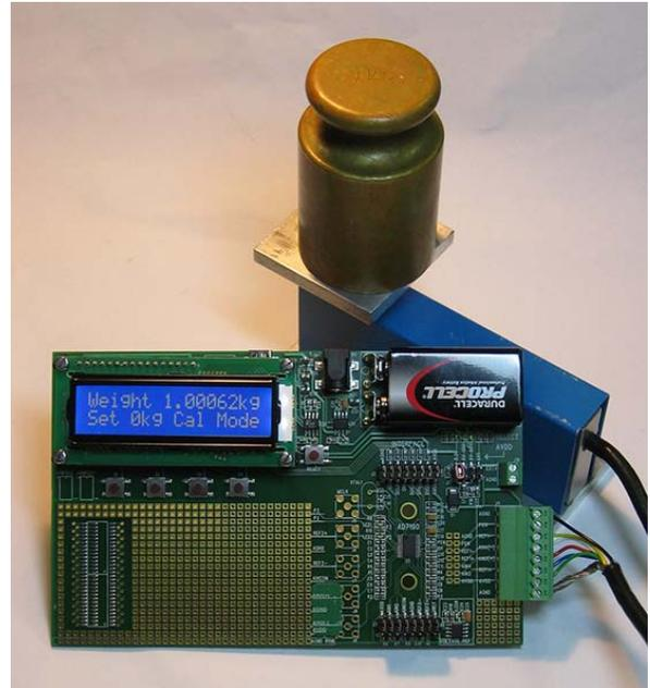
Figure 2. Weigh Scale System Setup Using the AD7195
