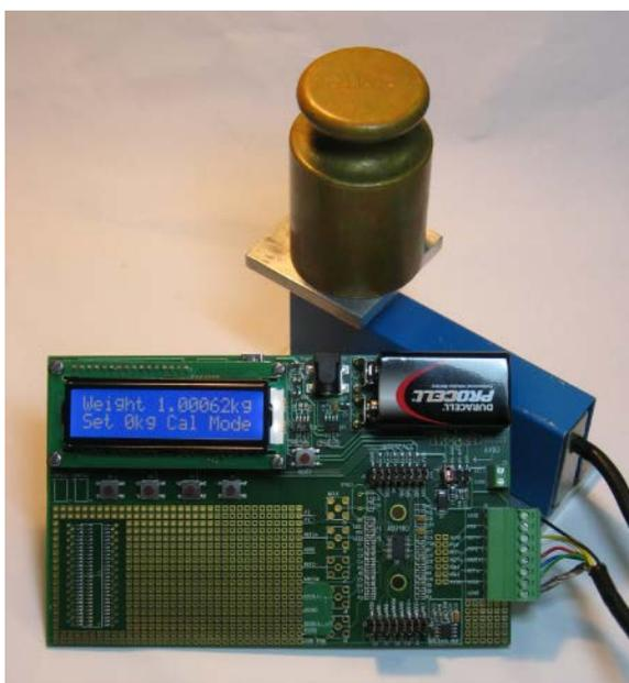
conversions are gathered. The noise of the system is calculated by the software to be 14 nV and is 98 nV peak-to-peak. This equates to 102,000 noise-free counts or 16.6 bits of noise-free code resolution.
