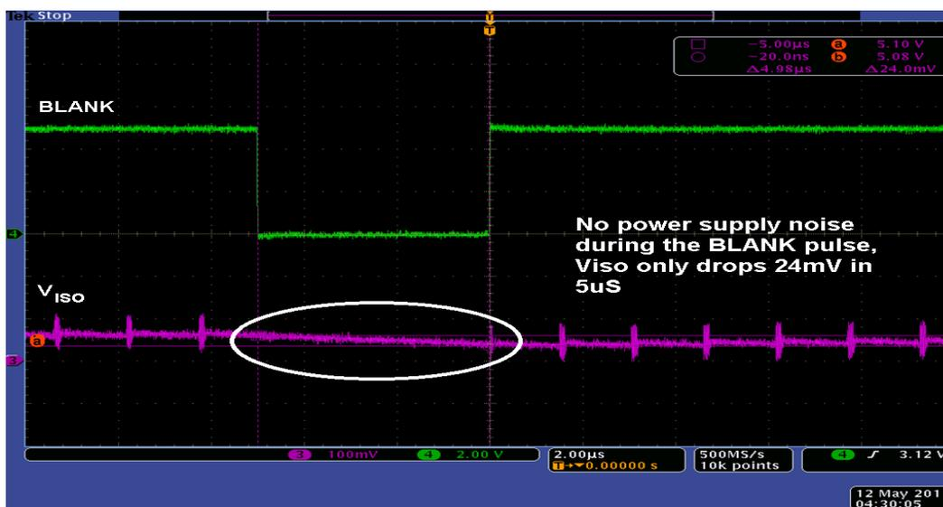
Figure 4. Full Operation with a 10 mA Load and 24 mV Supply Sag Due to the BLANK Pulse
