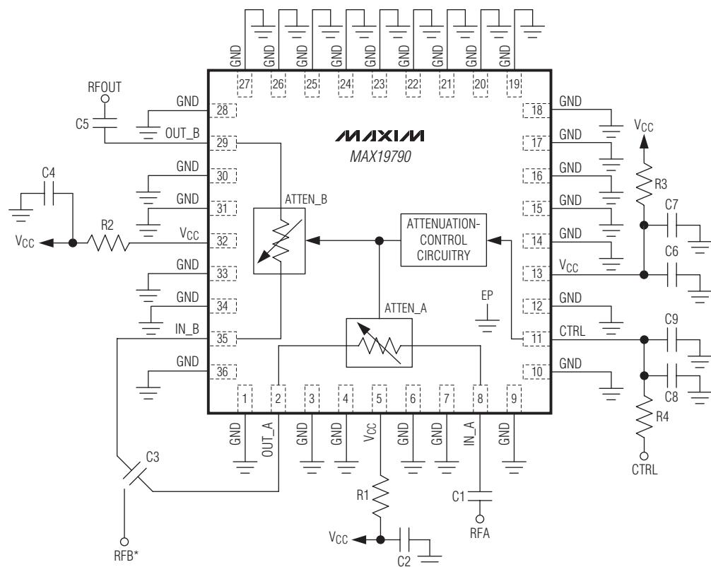
\*SCHEMATIC SHOWS CONFIGURATION FOR TWO CASCDED ATTENUATORS. TO USE ATTENUATOR A ONLY MOVE C3 TO CONNECT OUT\_A TO RFB. TO USE ATTENUATOR B ONLY MOVE C3 TO CONNECT RFB TO IN\_B.
