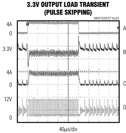
A. I_{OUT3} = 0.2A TO 4A , 5A/div B. V_{OUT3} = 3.3V , 100mV/div C. INDUCTOR CURRENT, 5A/div D. LX3, 10V/div \overline{SKIP} = GND
