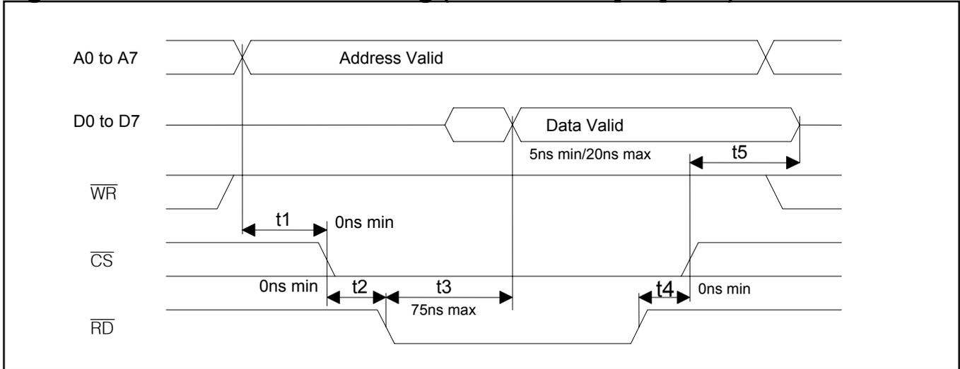
**Figure 19-5. Intel Bus Write Timing (BTS = 0 / BIS[1:0] = 01)**
