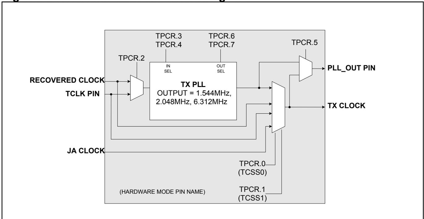
Figure 3-4. Master Clock PLL Diagram
