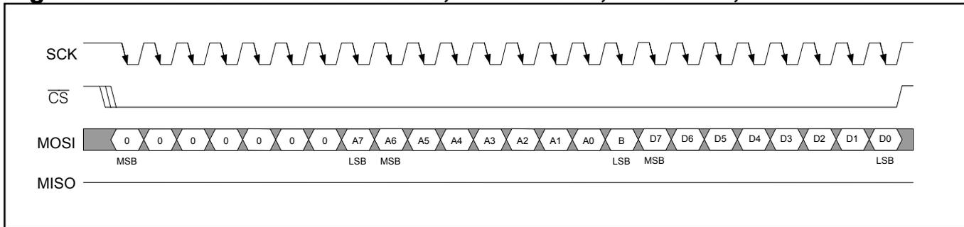
**Figure 17-7. SPI Serial Port Access, Write Mode, CPOL = 0, CPHA = 1**
