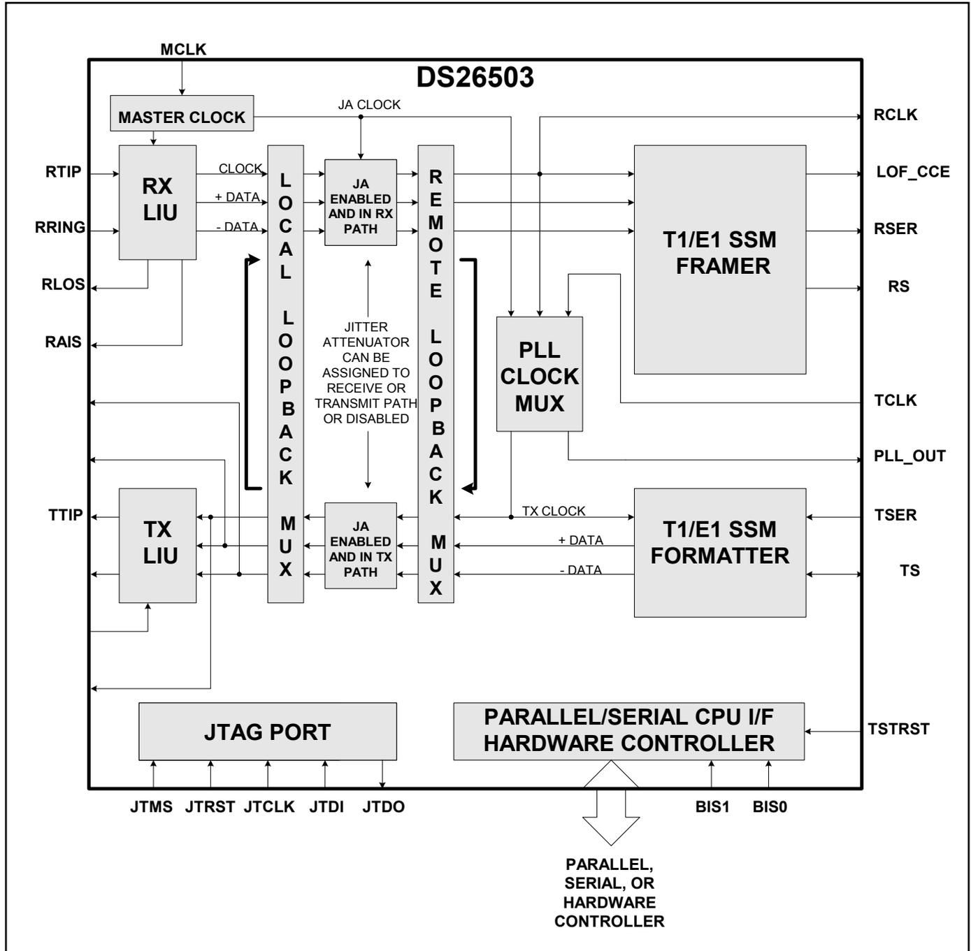
**Figure 3-2. Loopback Mux Diagram (T1/E1 Modes Only)**
