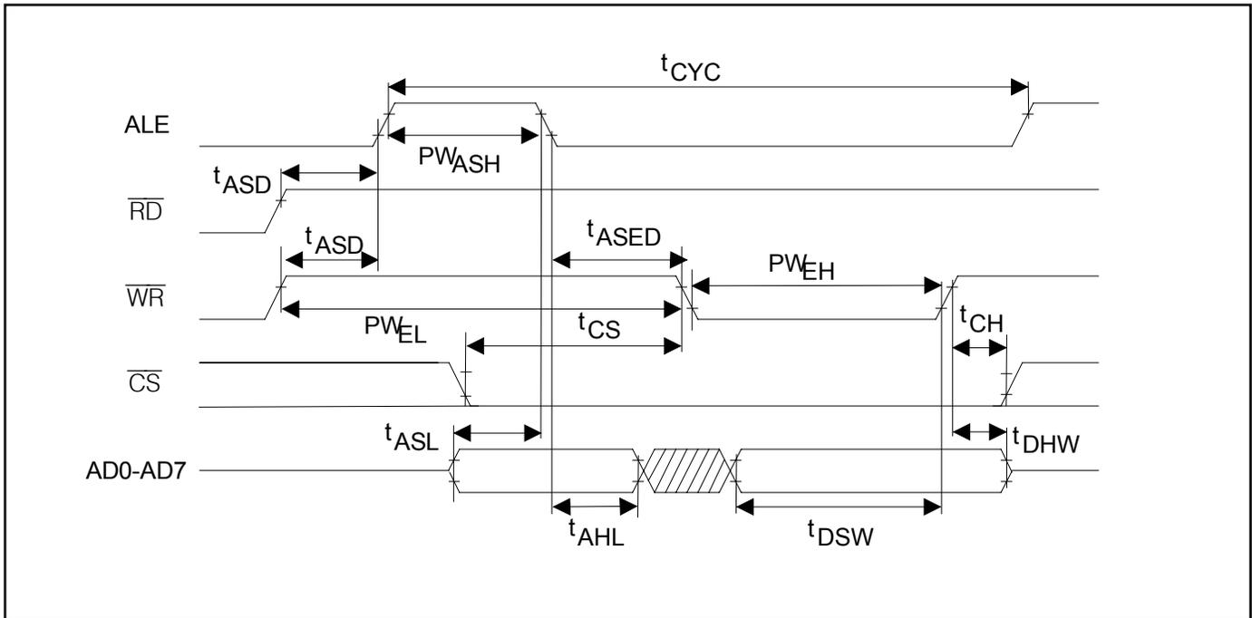
**Figure 19-3. Motorola Bus Timing (BTS = 1 / BIS[1:0] = 00)**
