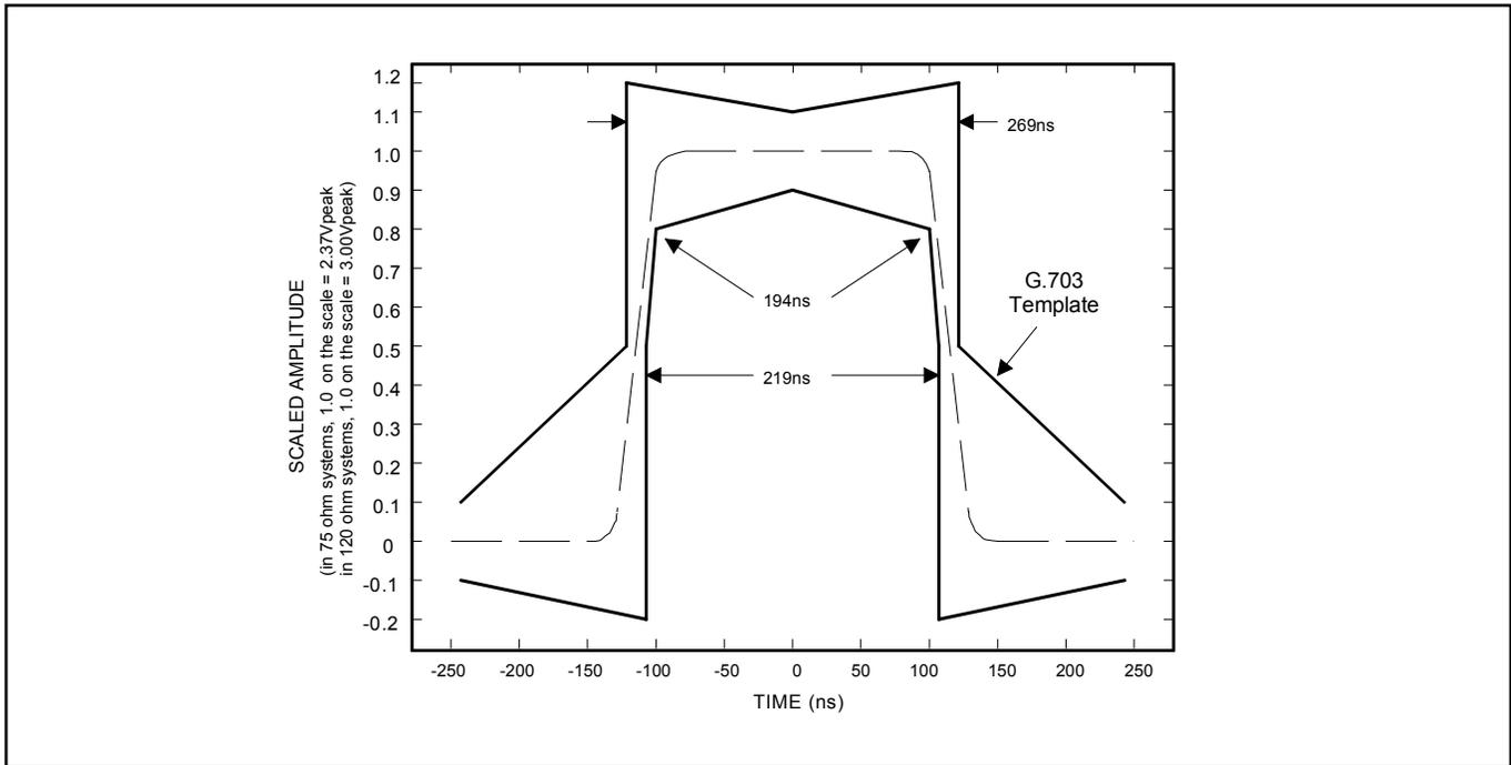
Figure 13-7. T1 Transmit Pulse Template
