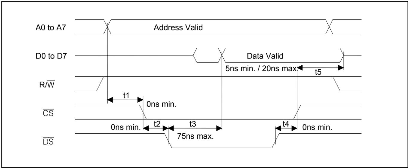
**Figure 19-7. Motorola Bus Write Timing (BTS = 1 / BIS[1:0] = 01)**
