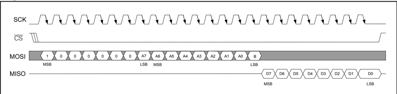
**Figure 17-4. SPI Serial Port Access, Read Mode, CPOL = 1, CPHA = 1**
