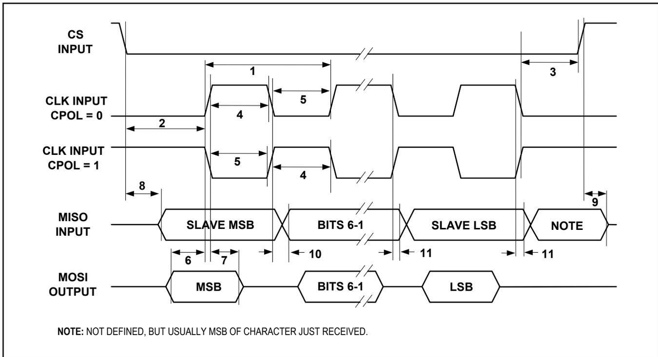
**Figure 19-9. SPI Interface Timing Diagram, CPHA = 1, BIS[1:0] = 10**
