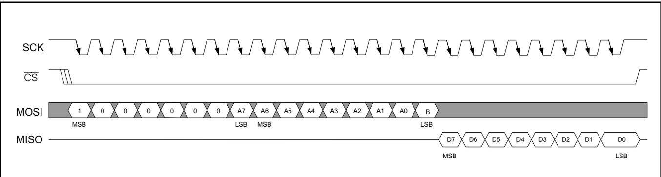
**Figure 17-3. SPI Serial Port Access, Read Mode, CPOL = 0, CPHA = 1**
