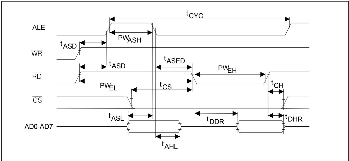
**Figure 19-2. Intel Bus Write Timing (BTS = 0 / BIS[1:0] = 00)**
