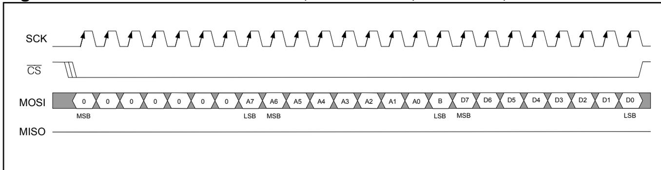
**Figure 17-6. SPI Serial Port Access, Write Mode, CPOL = 1, CPHA = 0**
