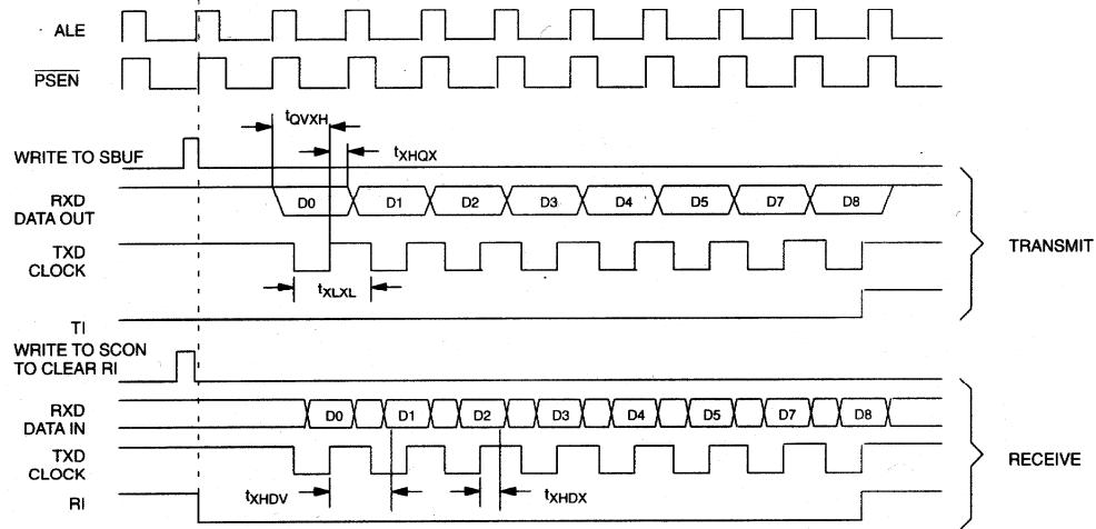
SERIAL PORT 0 (SYNCHRONOUS MODE)
