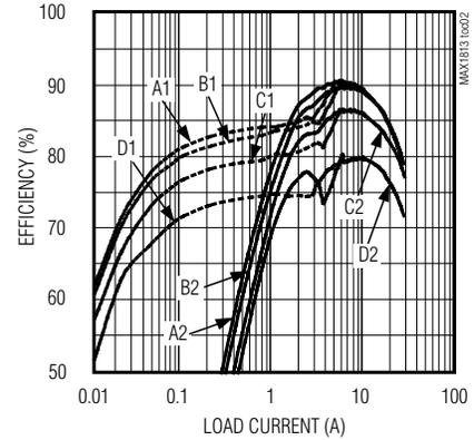
EFFECTIVE EFFICIENCY vs. LOAD CURRENT
