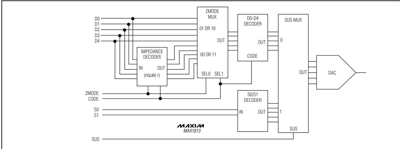
Figure 6. Internal Multiplexers Block Diagram
