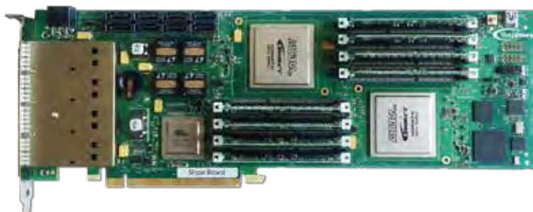
Dual Intel® Stratix V GX/GS PCIe Board with Quad QSFP+, DDR3, QDRIL+ and RLDRAM3
