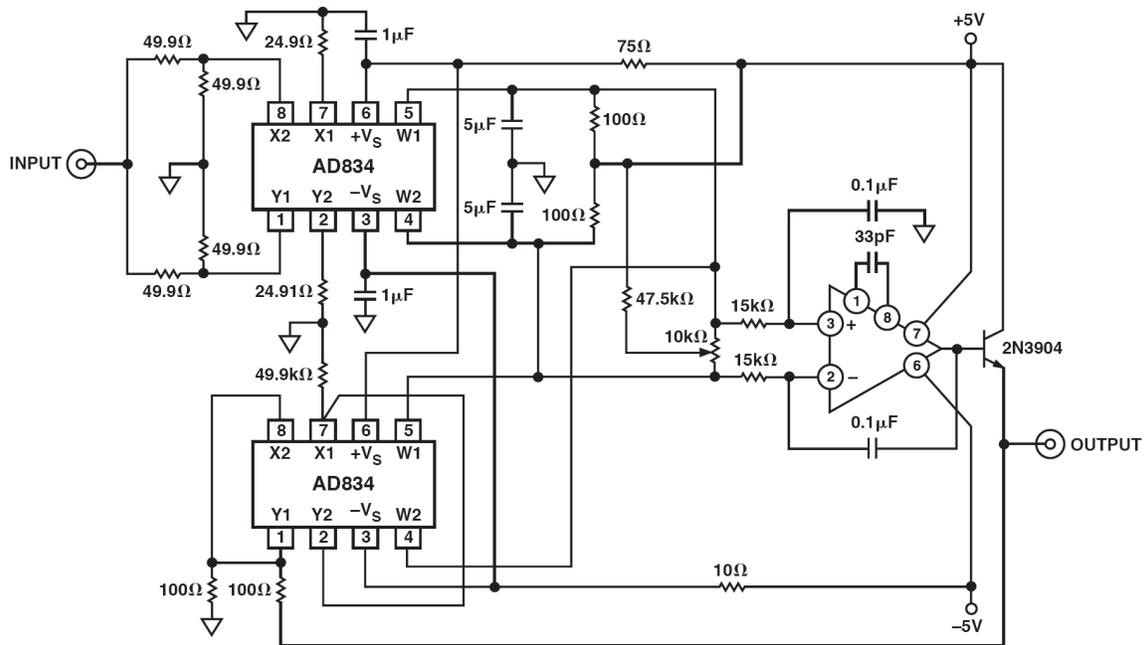
**Figure 2: Wideband RMS Measurement with the AD834 Analog Multiplier**
