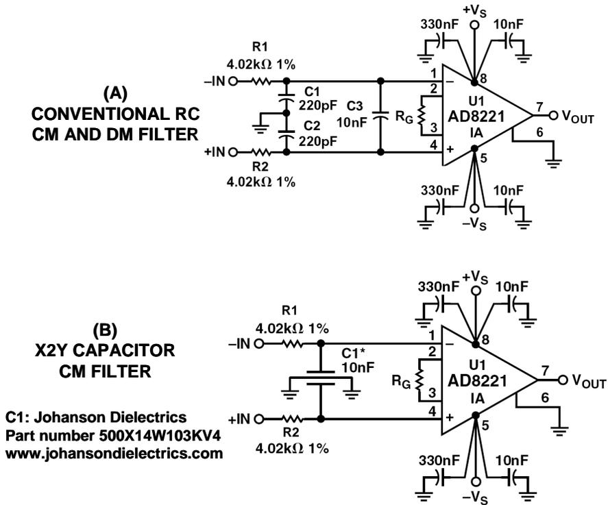
Figure 5: Conventional RC and X2Y CM Filters
