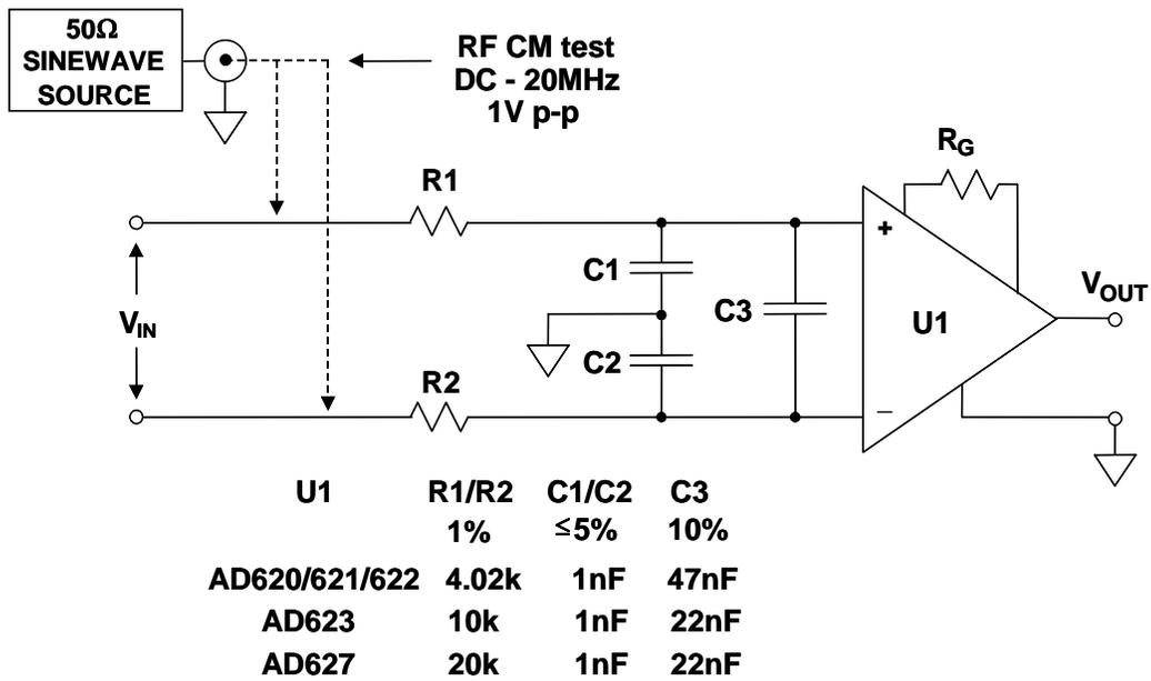
Figure 2: Flexible Common-Mode and Differential-Mode RC EMI/RFI Filters are useful with the [AD620](#) Series, the [AD623](#), [AD627](#), and other In-Amps
