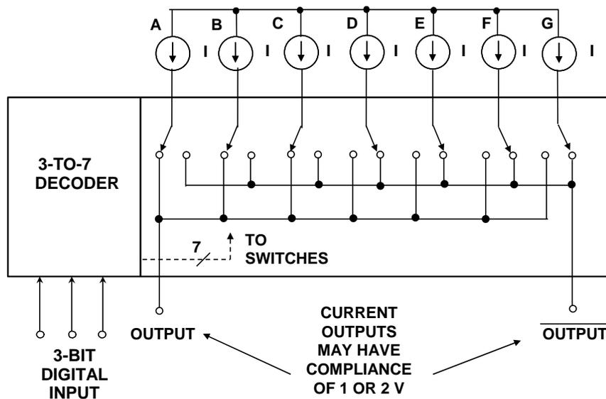
**Figure 6: High Speed Thermometer DAC with Complementary Current Outputs**
