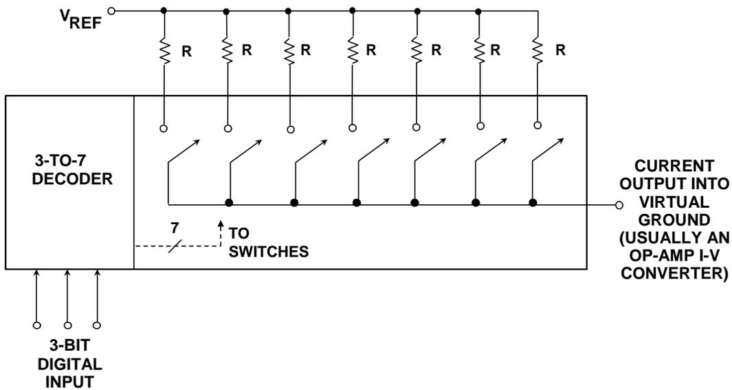
**Figure 4: The Simplest Current-Output Thermometer (Fully-Decoded) DAC**
