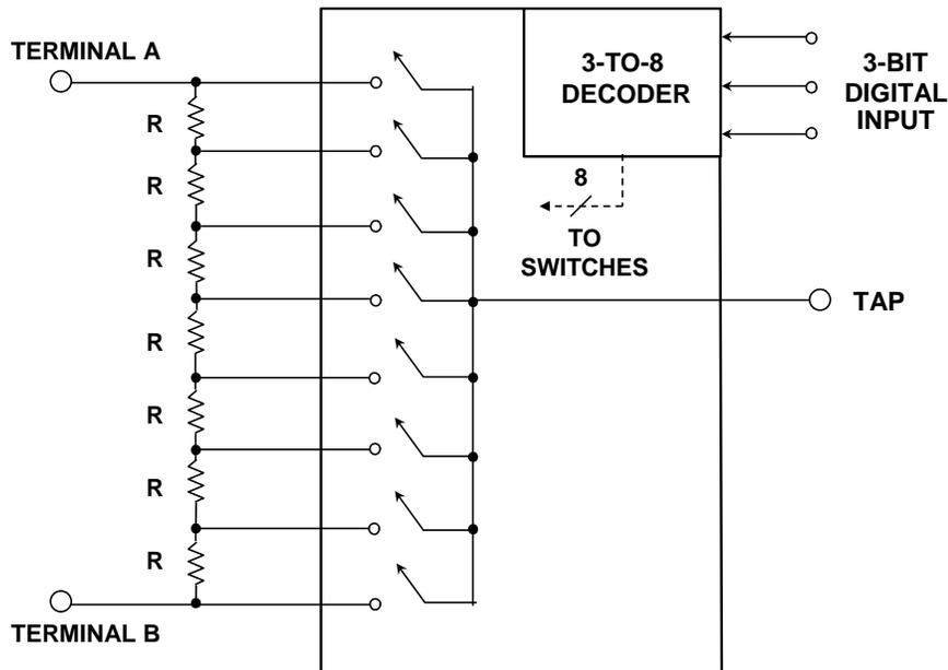
**Figure 3: A Slight Modification to a String DAC Yields a "Digital Potentiometer"**
