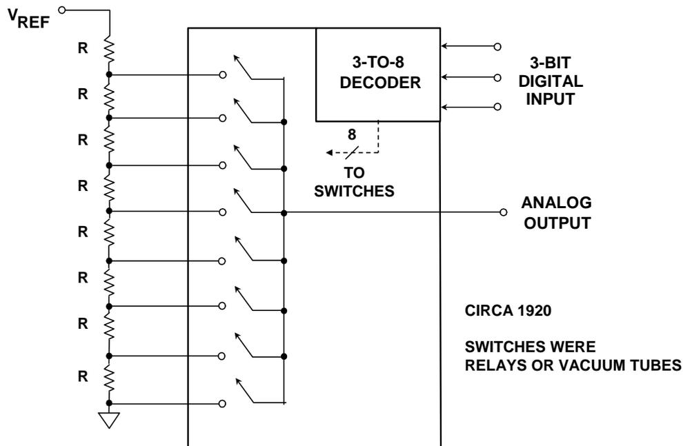
**Figure 2: Simplest Voltage-Output Thermometer DAC:
