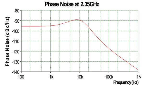
Figure 8. Closed loop phase noise simulation at 2.35 GHz
