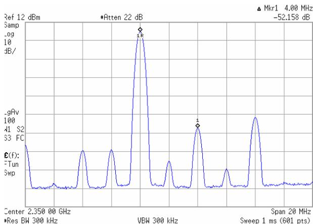
Figure 5. I/Q DC offset correction and sideband nulling.
