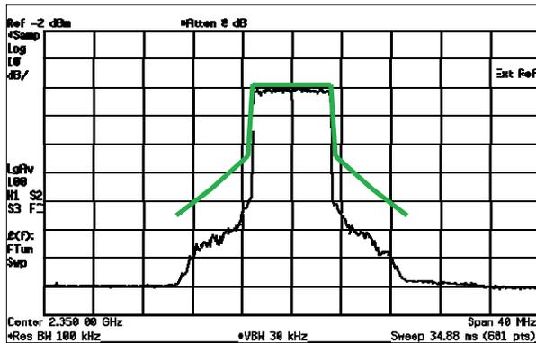
Figure 12. Spectral quality at 2.35GHz
