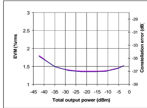
Figure 13. EVM function of gain control
