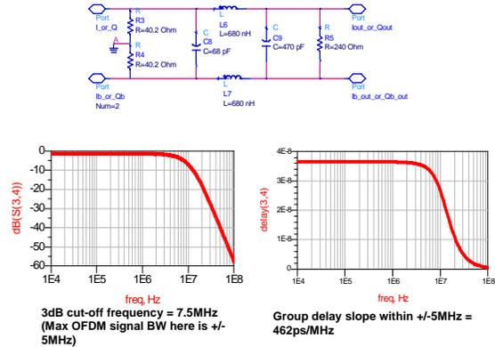
Figure 3. Baseband Bessel Low Pass Filter
