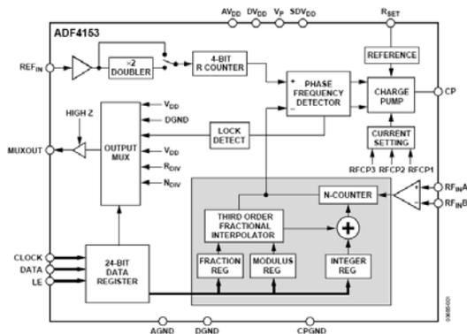
Figure 7. ADF4153 4 GHz Fractional-N Synthesizer. A simple 3-wire interface controls all on-chip registers. The device operates with a power supply ranging from
