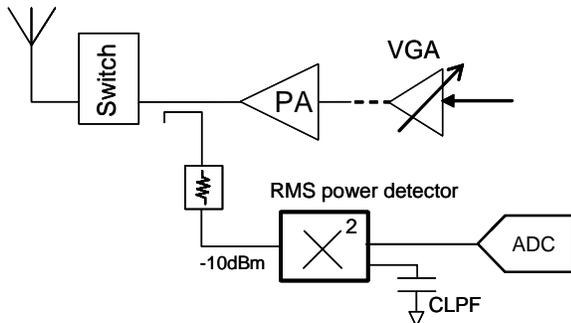
Figure 11. Power detection Circuit
