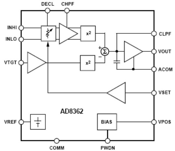
Figure 10. AD8362 50 Hz to 2.7 GHz 60 dB TruPwr™ Detector
