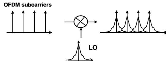
Fig 6. LO phase noise modulation of the OFDM subcarriers
