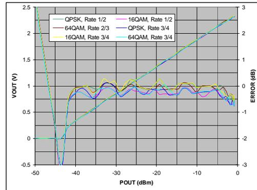
Figure 14. AD8362 RMS Detector Output Voltage and linearity error vs. System Output Power and Signal Type
