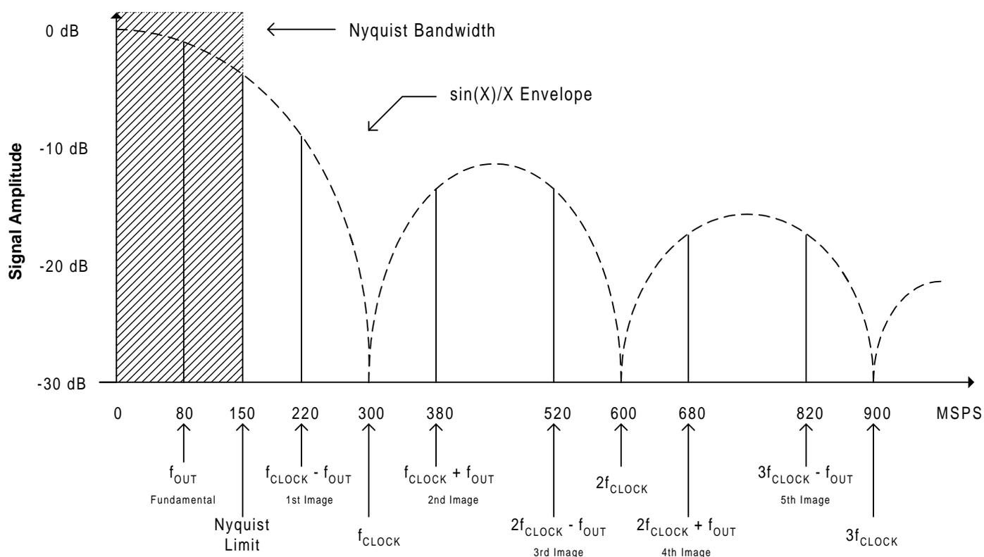
Figure 2-1. Spectral Analysis of Sampled Output
