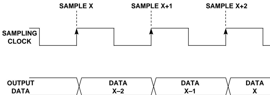
ABOVE SHOWS TWO CLOCK-CYCLES PIPELINE DELAY
