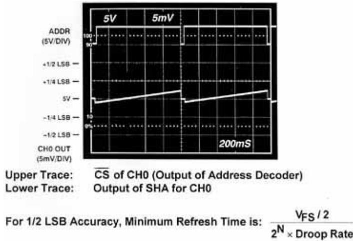
Where N is the DAC resolution in bits,  $V_{FS}$  is the DAC Full Scale Voltage
