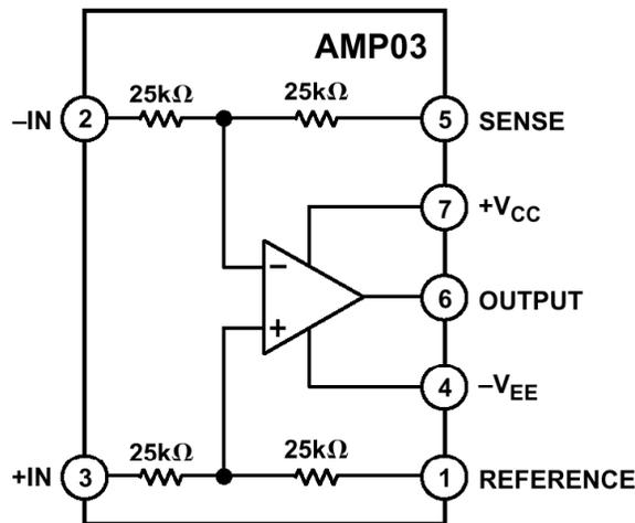
**Figure 2-3: AMP03 precision difference amplifier**
