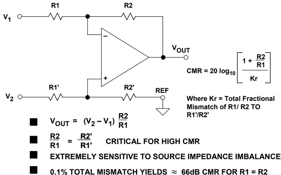
**Figure 2-2: Op amp subtractor or difference amplifier**
