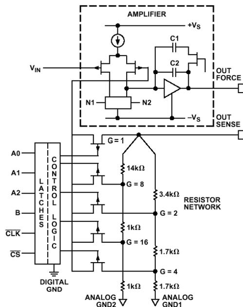
**Figure 2-37:** AD526 software programmable PGA simplified schematic
