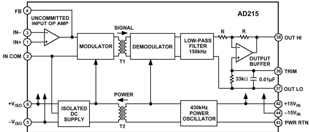
**Figure 2-51:** AD215 120kHz low distortion 2-port isolation amplifier
