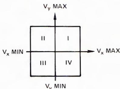
Figure 6. Input plane showing multiplication quadrants
