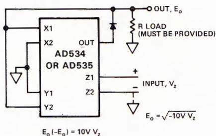
Figure 5. Connection of the AD534/AD535 for square rooting
