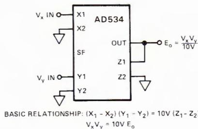
Figure 3. Signal connections of an actual multiplier
