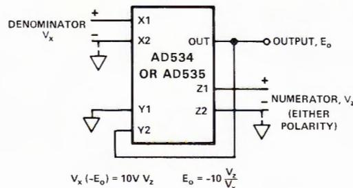
Figure 4. Connection of the AD534/AD535 for division
