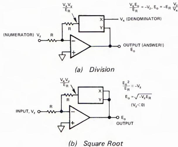
Figure 2. Feedback connection of conceptual multiplier for division and square-rooting
