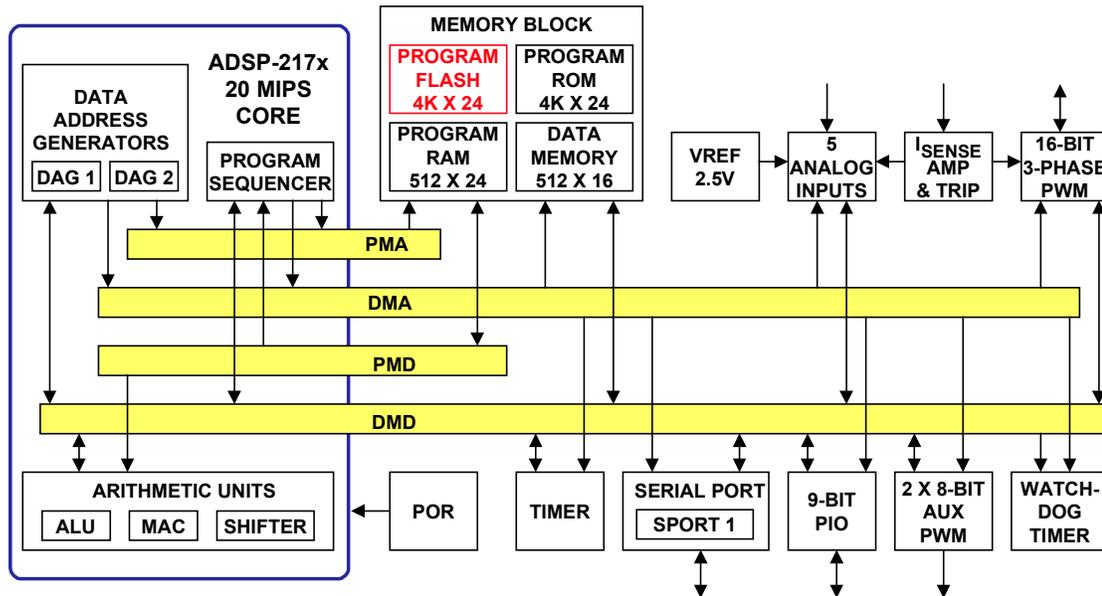
■ **New ADMCF5xx Family Based on ADSP-219x 150 MIPS Core with 128K Bytes Flash Memory**
