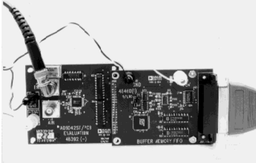
Using this hardware and Windows-based software to capture the ADC data, many testing possibilities exist. Figure 7.23 shown a time-domain plot of data captured using the fifo memory. Once the data is captured, FFT analysis (Figure 7.24) or DNL histograms (Figure 7.25) are easily generated.
