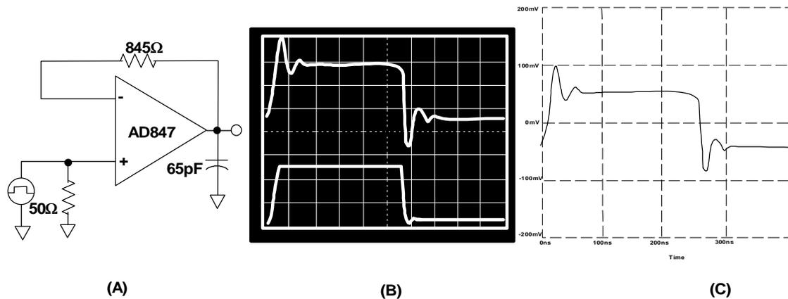
Properly laid out PC board and simulation agree closely
