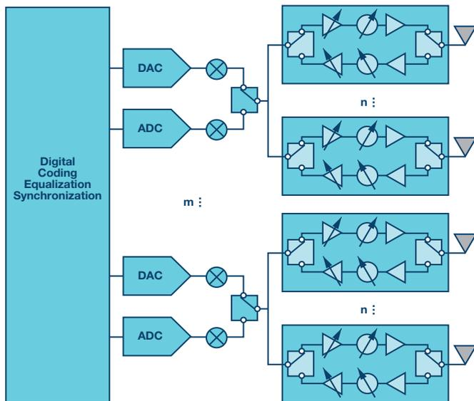
Figure 1. Hybrid beamforming block diagram.
