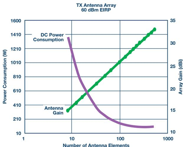
Figure 3. Antenna gain vs. the power dc power consumption of the Tx section of the antenna.
