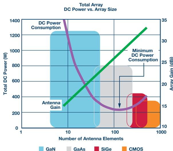
Figure 4. DC power consumption of entire antenna array vs. antenna gain.
