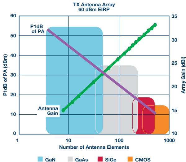
Figure 2. Antenna gain vs. output level requirement of power amplifier.
