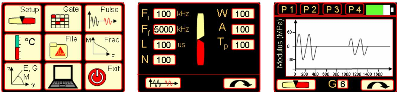
**Figure 6. The clearly designed user interface with a main menu (left), parameter settings (middle) and signal graphics (right) conceals the complexity of the system**
