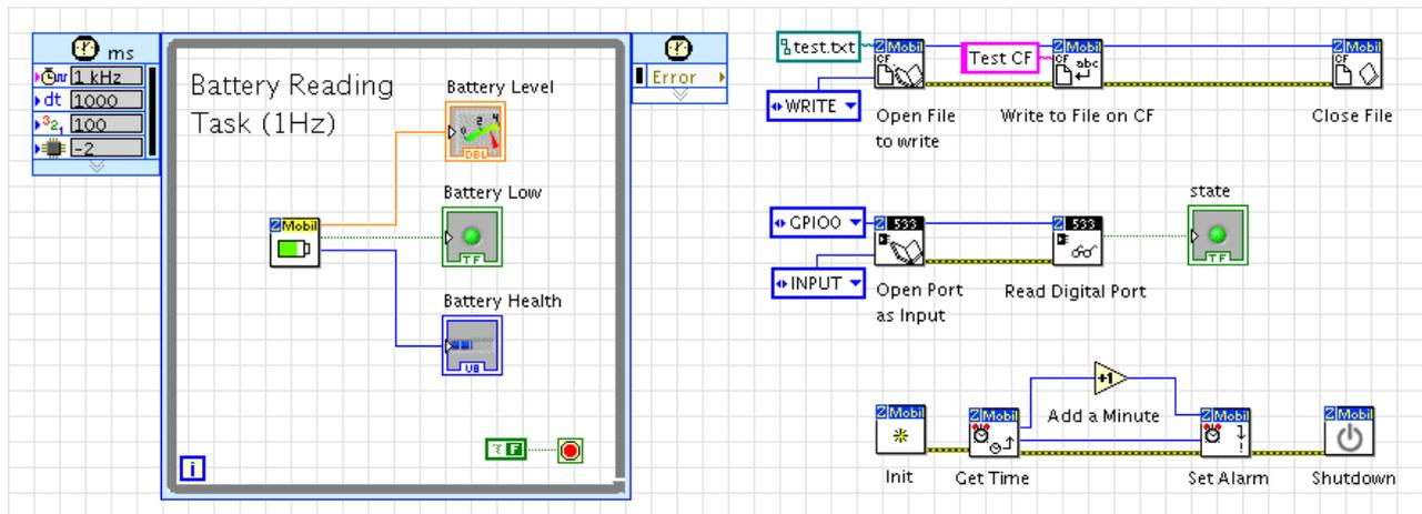
**Figure 5. Programming model of the ZMobile embedded platform: battery monitoring (left), alarm and shutdown (right bottom), digital IO (right middle) and reading/writing to removable memory such as a CF card (right top)**
