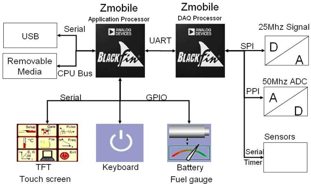
**Figure 2. Block diagram with application processor (left) and separate co-processor for data acquisition and signal analysis (right).**
