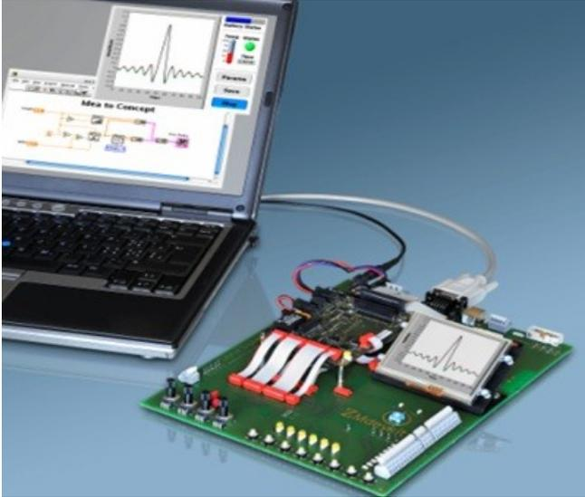
**Figure 7. The ZMobile Development Kit (Schmid Engineering) offers an easy introduction to program with LabVIEW Embedded**
