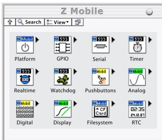
Figure 4. Graphical embedded system programming "Out-of-the-Box" with standardized function blocks /VIs.
