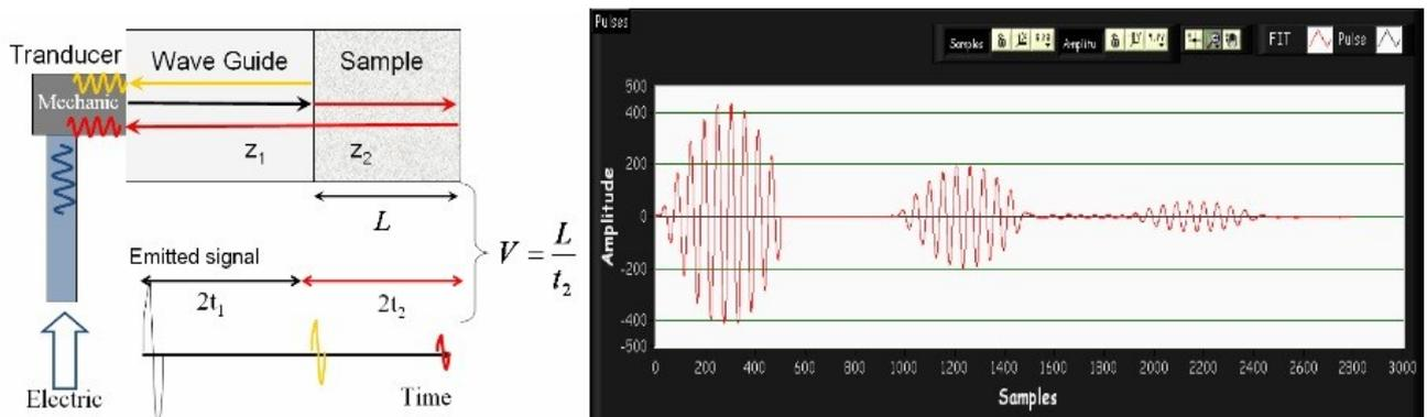
**Figure 3. Left: an electric signal is converted to a mechanical signal with a transducer. The generated ultrasonic wave propagates through the material where it is submitted to a reflection at the interface between the wave guide and the sample. Right: the time of fly is acquired with the embedded oscilloscope.**
