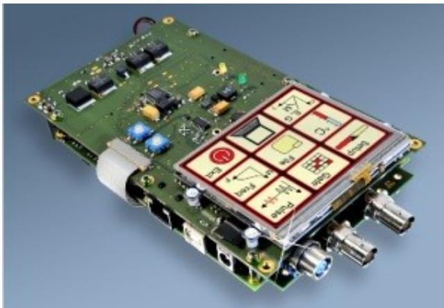
**Figure 8. Measurement handheld under the hood: Stacked construction in combination with standard OEM modules and application specific boards.**
