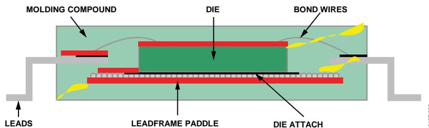
Figure 69. Package Cross Section Showing Delamination (Red) and Cracking (Yellow)
