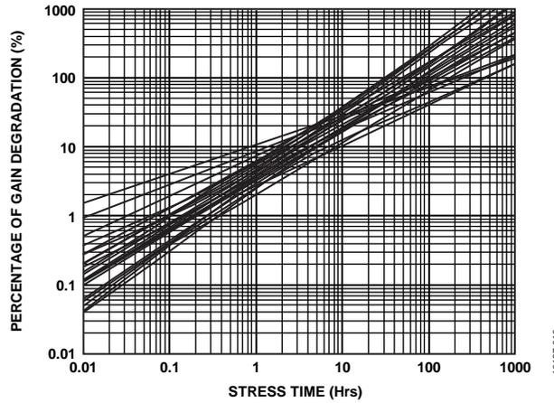
Figure 28. Graph of % Gain Degradation vs. Stress Time
