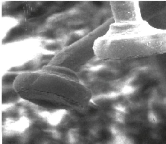
Figure 83. Lifted Ball Bonds after Extended Temperature Cycle
