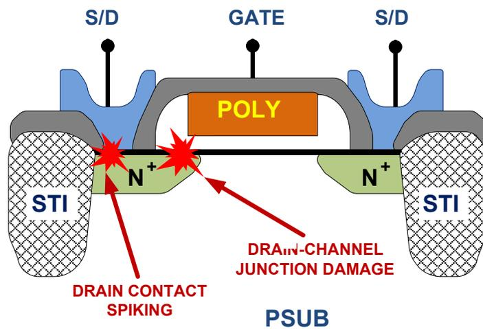
Figure 111. Locations of Typical HBM Contact Spiking and Junction Damage
