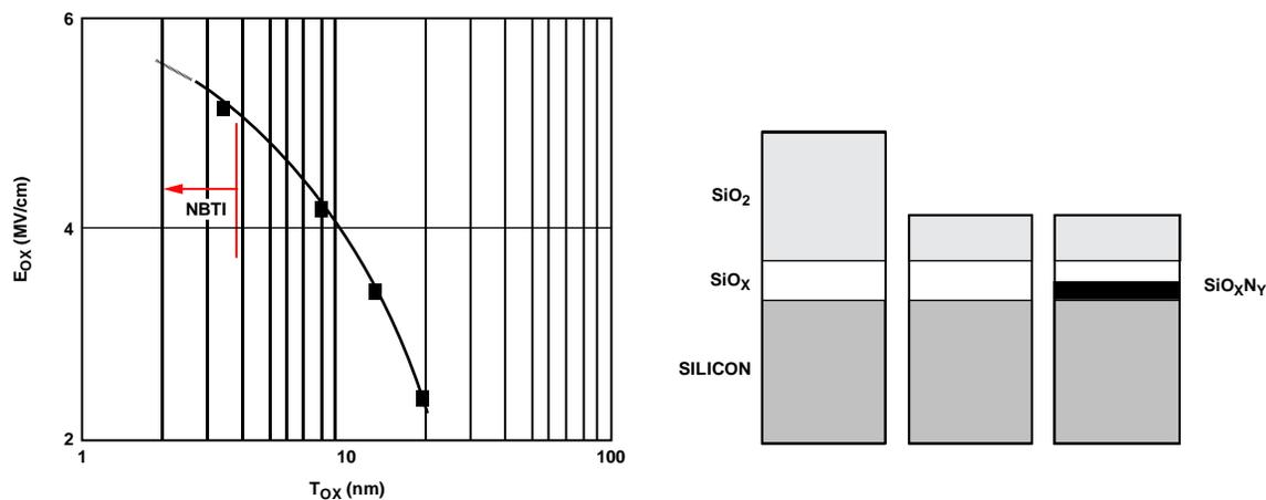
Figure 36. Shrinking Geometries and Increasing E-Fields
