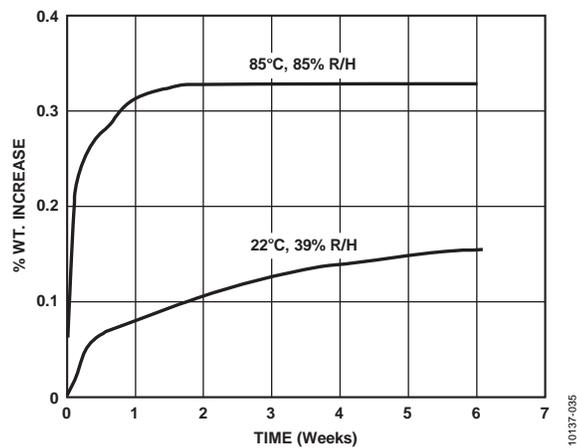
Figure 66. Moisture Absorption Graphs for a 44 PLCC Package at Various Conditions
