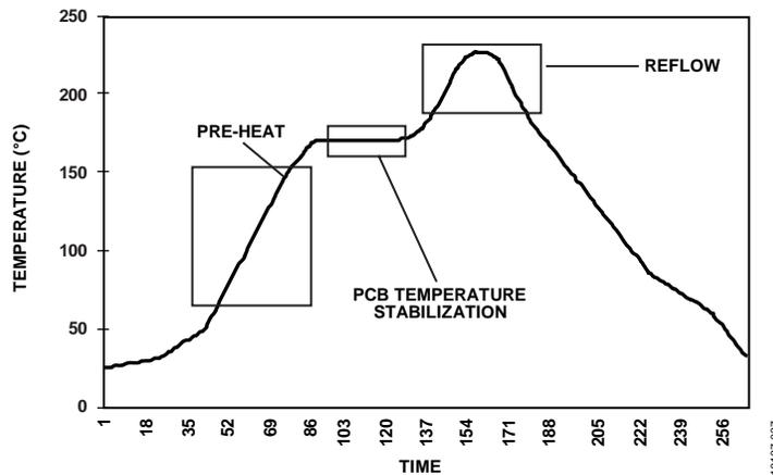
Figure 68. Typical Solder Profile
