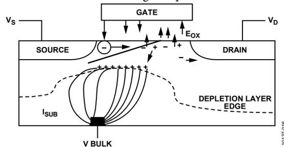
Figure 22. Hot Electron Injection
