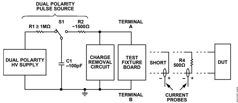
Figure 102. HBM ESD Test Circuit (Excerpted from ANSI/ESDA/JEDEC JS-001-2011)
