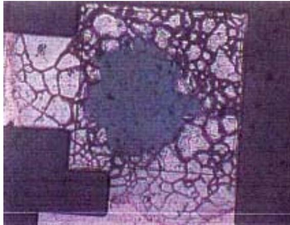
Figure 75. Corroded Bond Pad
