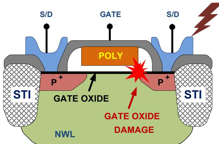
Figure 109. Location of Typical FICDM Gate Oxide Damage
