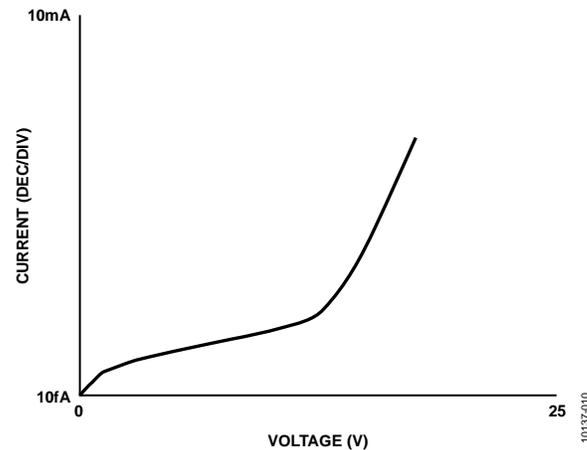
Figure 13. Dielectric Breakdown Curve
