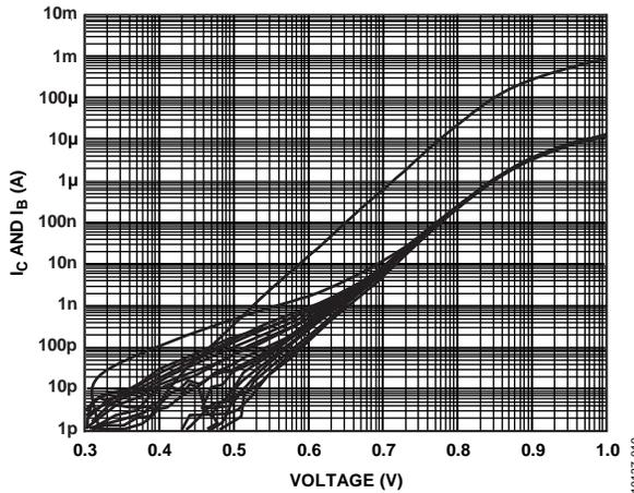
Figure 29. Gummel Plot  $I_C$  (Upper Curve) and  $I_B$  (Lower Curve) vs. Voltage
