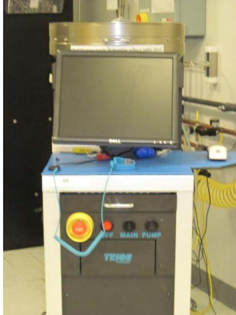
Figure 132. Reactive Ion Etcher
