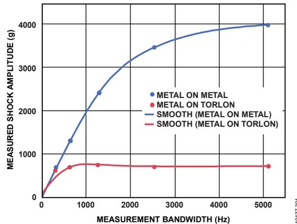
Figure 101. Shock Amplitude vs. Analysis Bandwidth, 38 mm Drop Height
