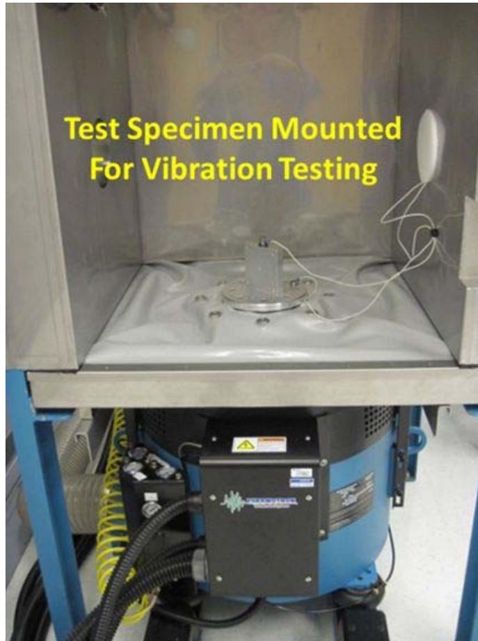
Figure 95. Thermotron DSX-2250 Temperature/Vibration System
