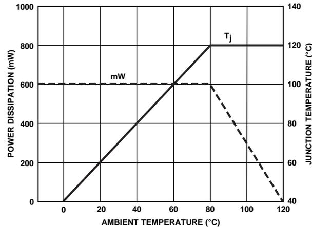
Figure 63. Power Dissipation (mW) and Junction Temperature (°C) vs. Ambient Temperature
