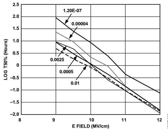
Figure 15. T50% Failure Time vs. Electric Field
