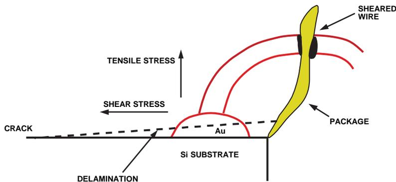
Figure 81. Bond Wire Shearing as a Result of Microcracks
