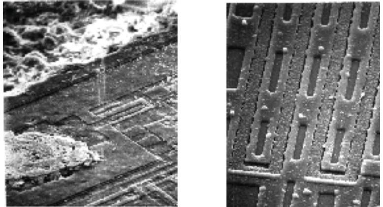
Figure 78. Imprints of the Die on the Plastic Molding Compound After Processing
