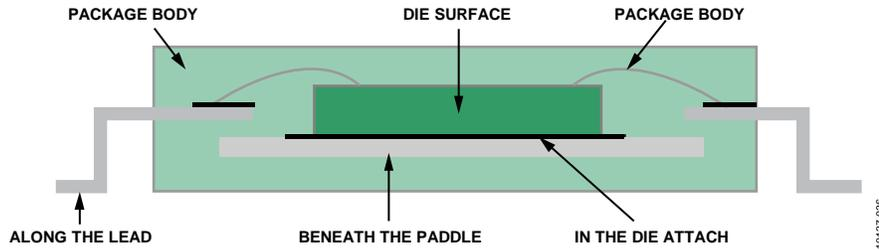
Figure 67. Cross Section of a Typical Package
