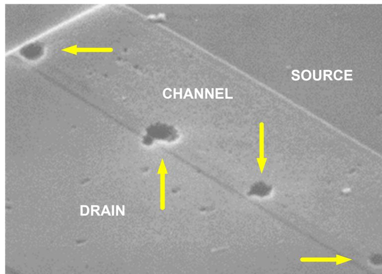
Figure 110. Scanning Electron Microscope (SEM) Image Post Deprocessing to the Silicon Level Showing 4 Pits on a Sample Stressed at  $\pm 1,500$  V FICDM
