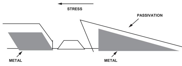
Figure 84. Metal Deformation Due to Shear Stress
