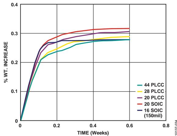
Figure 65. Moisture Absorption Graph for Various Packages at 85°C and 85% R/H
