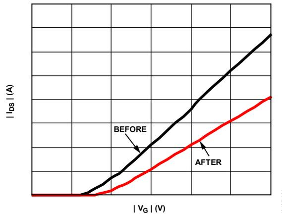
Figure 33. NBTI Degradation Mechanism
