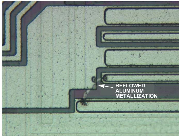
Figure 115. Optical Microscope Image of EOS Damage at a Bipolar Output Transistor
