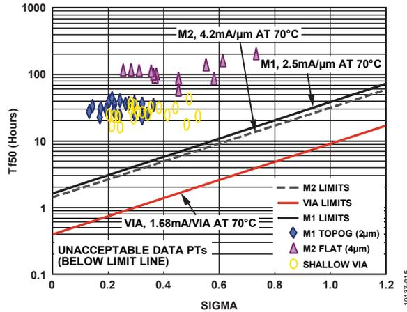
Figure 18. Selection of EM Monitor Results from a 0.6 μm Process
