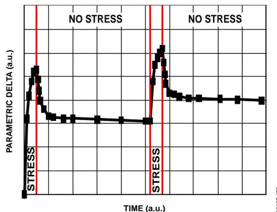
Figure 41. Permanent and Recoverable Degradation
