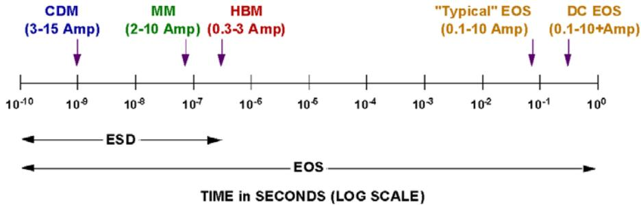
Figure 113. Spectrum Showing the Duration of Common EOS/ESD Events
