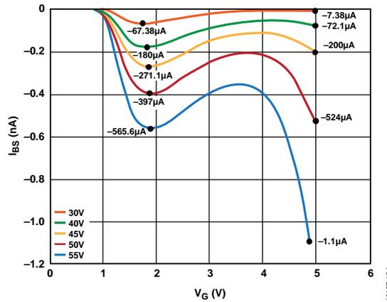
Figure 26. 40 V HVDMOS  $I_{BS}/V_{GS}$  Characteristics Plotted as a Function of  $V_{DS}$
