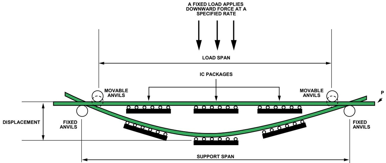
Figure 92. PCB Bend Testing Schema
