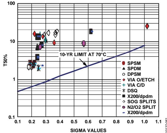
Figure 55. Gate Dielectric Reliability During Process Development
