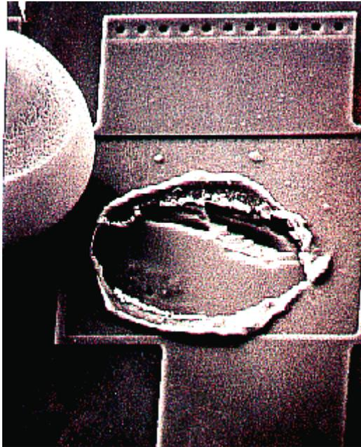
Figure 82. Bond Pad after Lifted Bonds During Extended Temperature Cycle
