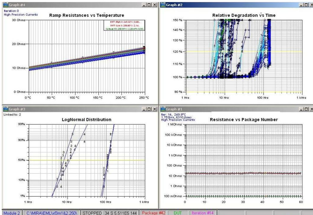
Figure 19. EM Testing and Analysis
