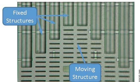
Figure 99. Vertical Stiction: Moving Structure is Stuck to the Substrate (Note Fixed Structures Out of Focus)
