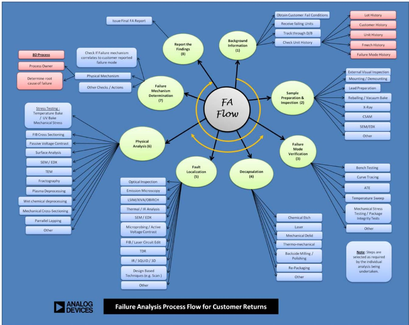
Figure 120. Failure Analysis Flow
