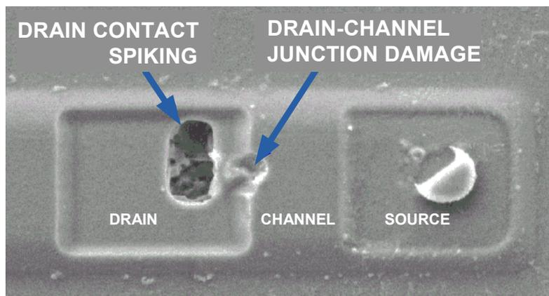
Figure 112. Scanning Electron Microscope (SEM) Image Post Deprocessing to the Silicon Level Showing Drain-to-Channel Junction Damage and Drain Contact Spiking on a Sample Stressed at ±2000 V HBM
