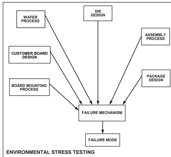
Figure 60. Process Interaction on Failure Mechanisms
