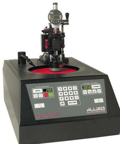
Figure 133. Parallel Polishing Tool
