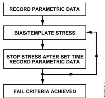
Figure 37. JEDEC NBTI Flow Chart
