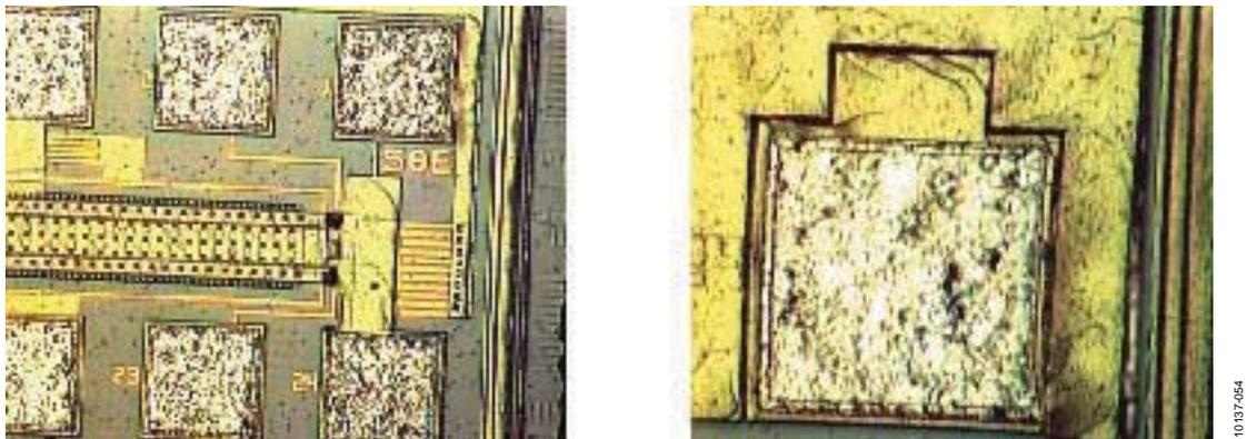
Figure 85. Metal Deformation as a Result of Shear Stress
