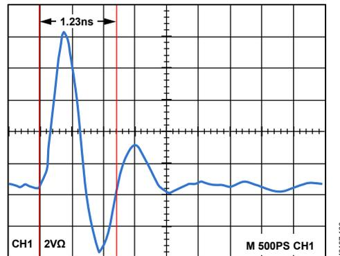
Figure 107. Field-Induced CDM ESD Current Waveform for a +250 V Discharge, Using a 30 pF Test Module and 3 GHz BW Oscilloscope (10 GS/s Sampling Rate); Note a Vertical Scale of 2 V/div Through a 1 $\Omega$  resistor = 2 A/div,  $I_{PEAK} \approx 9.6$  A, and a Horizontal Scale of 500 ps/div,  $T_{RISE}$  (10% to 90%  $I_{PEAK}$ )  $\approx 200$  ps.
