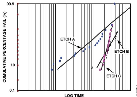
Figure 57. EM Lifetime Data for Various Etch Rates
