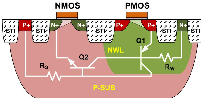
Figure 118. Cross Section and Schematic of Parasitic Bipolar Transistors in a Generic CMOS Process Technology Node
