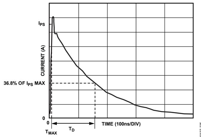
Figure 104. Current Waveform through a Shorting Wire ( $t_d$ )
