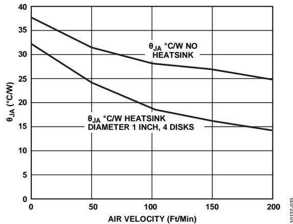
Figure 64.  $\theta_{JA}$  vs. Airflow
