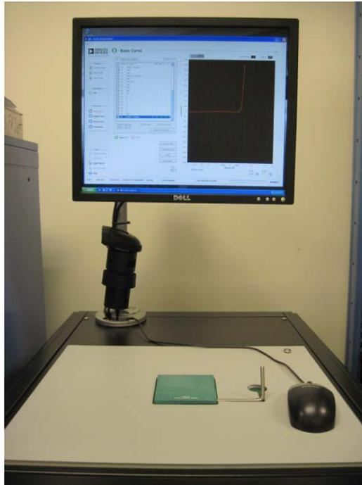
Figure 122. Automated Curve Tracer
