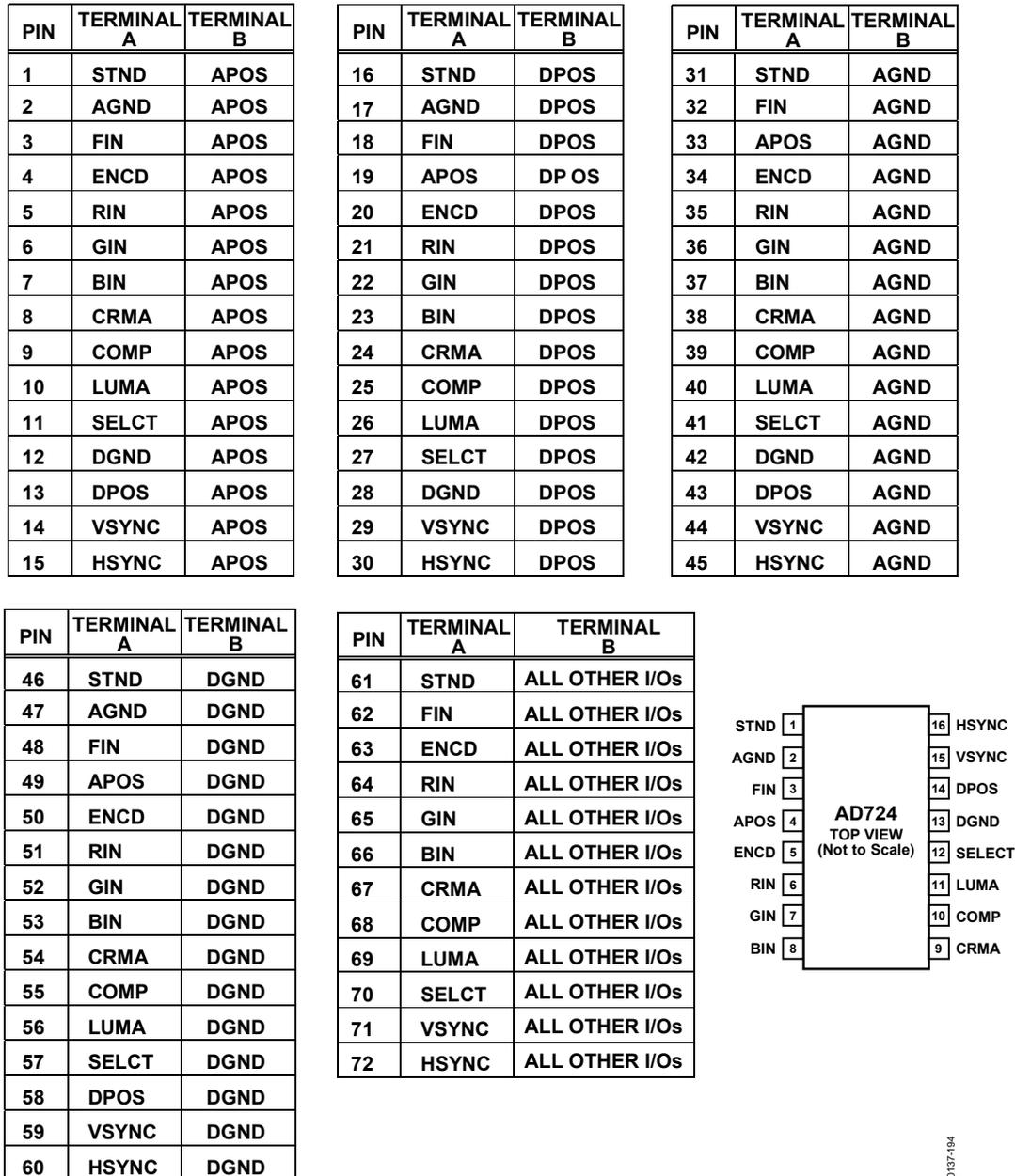
Figure 105. AD724 Pin Configuration and 72 Pin Combinations Zapped During AD724 HBM ESD Testing
