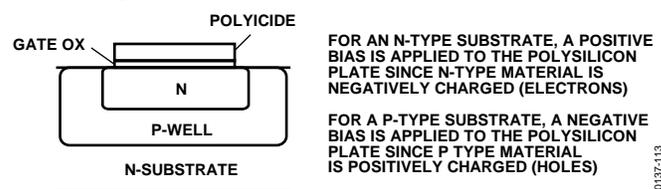
Figure 14. Testing in Accumulation
