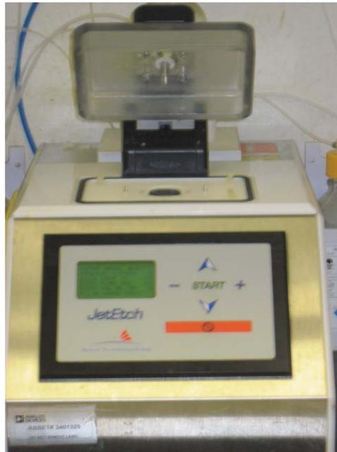
Figure 124. JetEtch Decapsulation Machine
