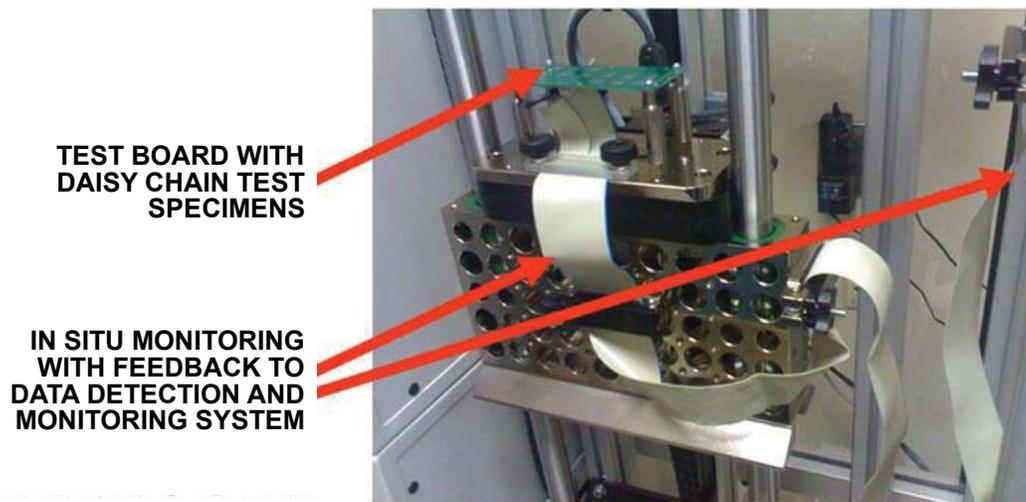
Figure 90. Mechanical Shock/Drop Test System
