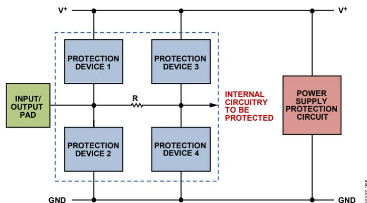
Figure 116. Generic On-Chip H-Network (in Dashed Blue Box)
