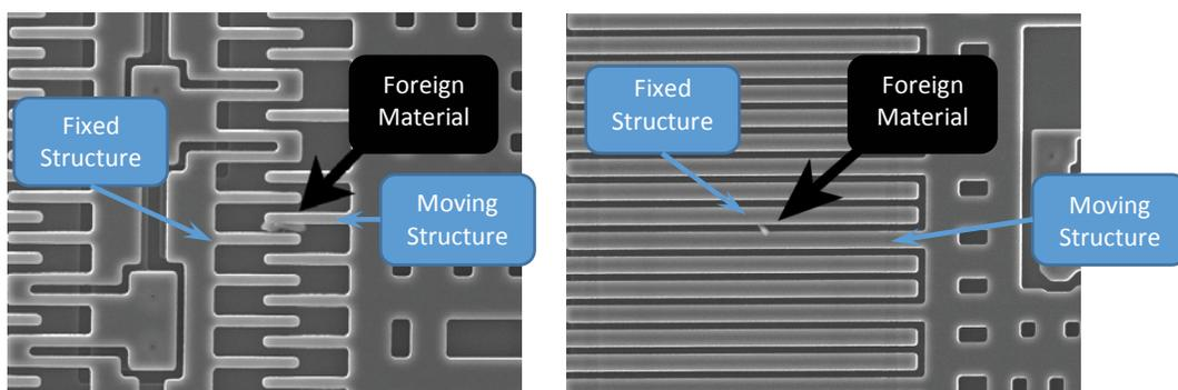
Figure 96. Foreign Material Impeding Sensor Motion
