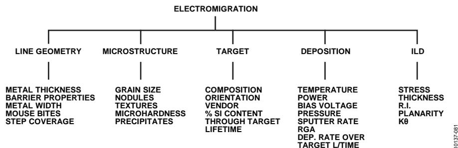
Figure 54. Section of Electromigration Flow Chart
