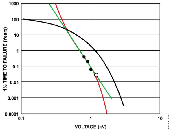
Figure 42. HV Lifetime Characteristic for Isolator Devices
