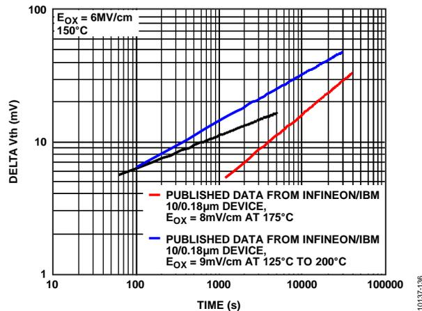
Figure 38. Delta V<sub>TH</sub> Proportional to Time
