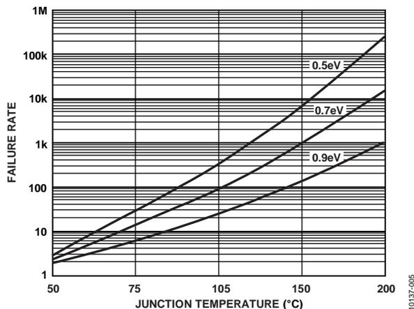
Figure 6. Failure Rate vs. Junction Temperature
