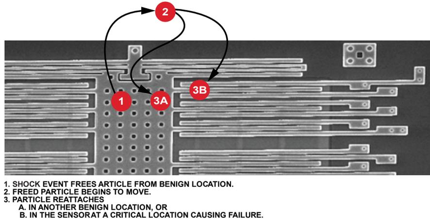
Figure 97. The Probabilistic Nature of the Foreign Material Failure Mechanism
