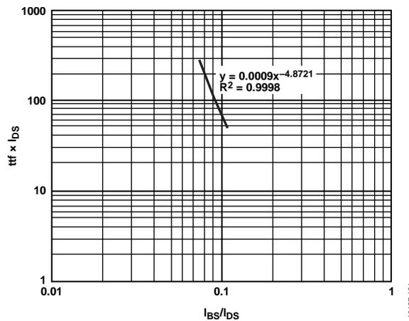
Figure 23. Typical Time to Failure vs.  $(I_{BS}/I_{DS})$  Curve for Hot Carrier Injection
