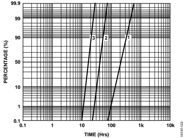
Figure 24. Cumulative Probability for Hot Carrier Degradation
