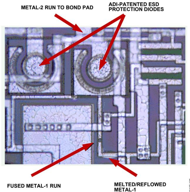
Figure 108. Optical Microscope Image of a 4  $\mu\text{m}$  Wide MET1 Interconnect on a Sample Stressed at  $\pm 2000$  V HBM
