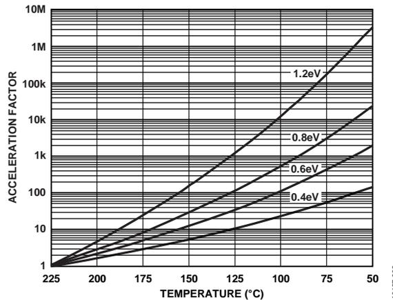
Figure 7. Acceleration Factor vs. Temperature
