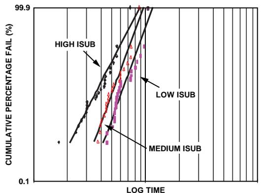
Figure 59. Hot Carrier Lifetimes and Their Relationship to Substrate Currents
