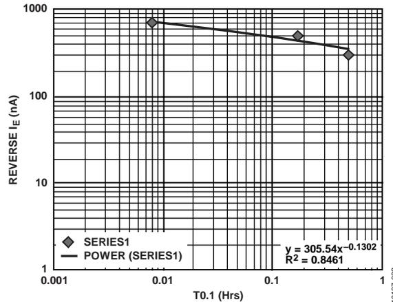
Figure 32. Lifetime vs. Reverse Bias  $I_E$
