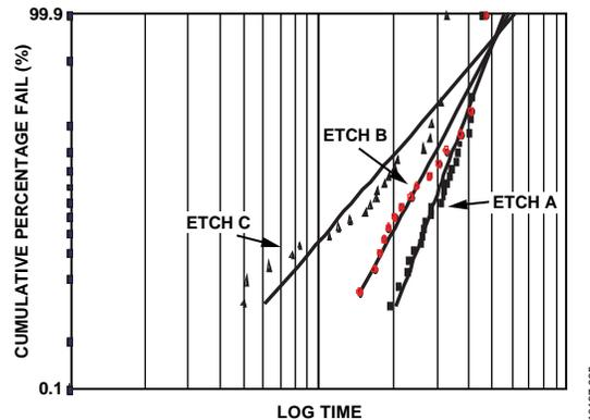
Figure 58. Hot Carrier Reliability vs. Different Via Etch Rates
