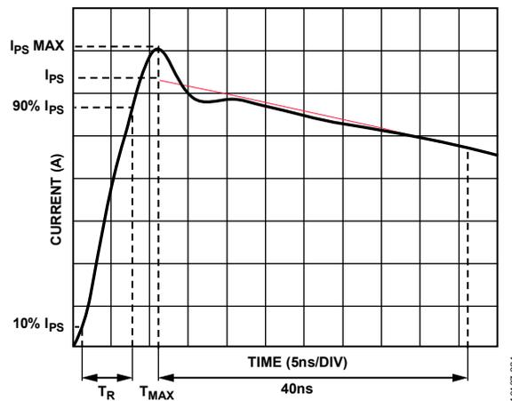
Figure 103. Current Waveform Through a Shorting Wire ( $I_{ps} \text{ MAX}$ )
