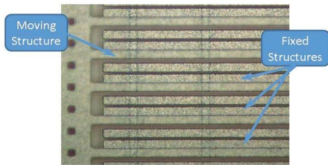
Figure 98. Lateral Stiction: Moving Structure is Stuck to Adjacent Fixed Structure
