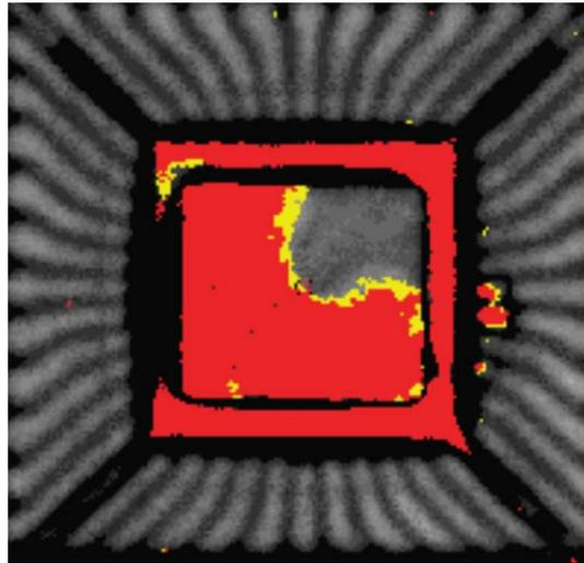
Figure 70. Acoustic Microscope Micrograph of a Delaminated 44 PLCC
