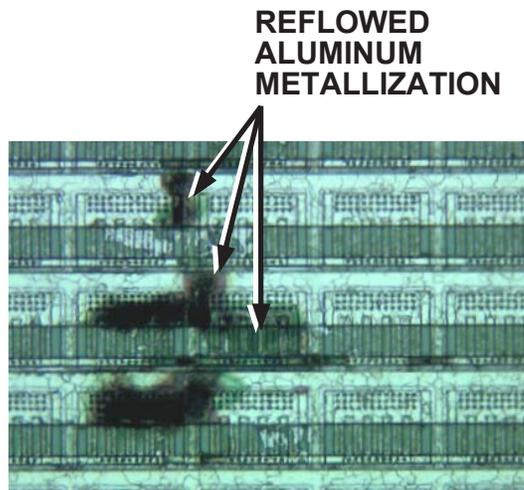
Figure 114. Optical Microscope Image of Severe Electrical Overstress (EOS)
