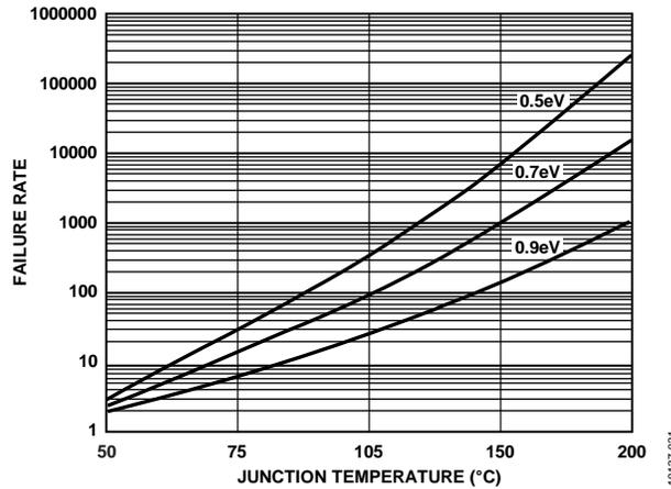
Figure 62. Failure Rate vs. Temperature (C)
