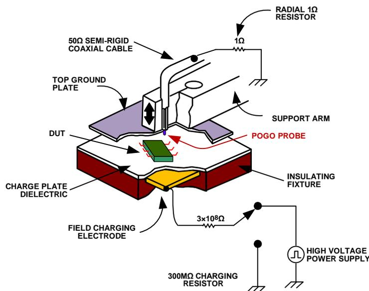
Figure 106. Field Induced CDM ESD Test Circuit (Excerpted from JEDEC Test Method JESD22-C101)
