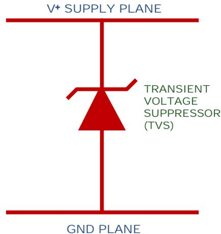
Figure 117. TVS Protection used for Protection Across Supply/Ground Planes in System Applications
