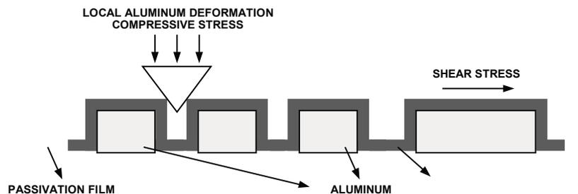
Figure 86. Metal Deformation Due to Filler Particles
