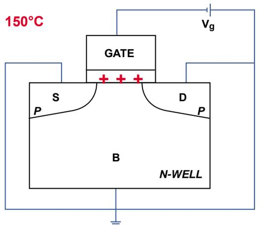
Figure 34. NBTI Bias Condition for pMOS
