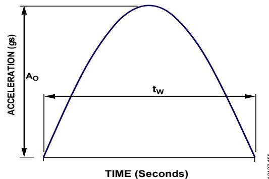
Figure 91. Mechanical Drop/Shock Profile
