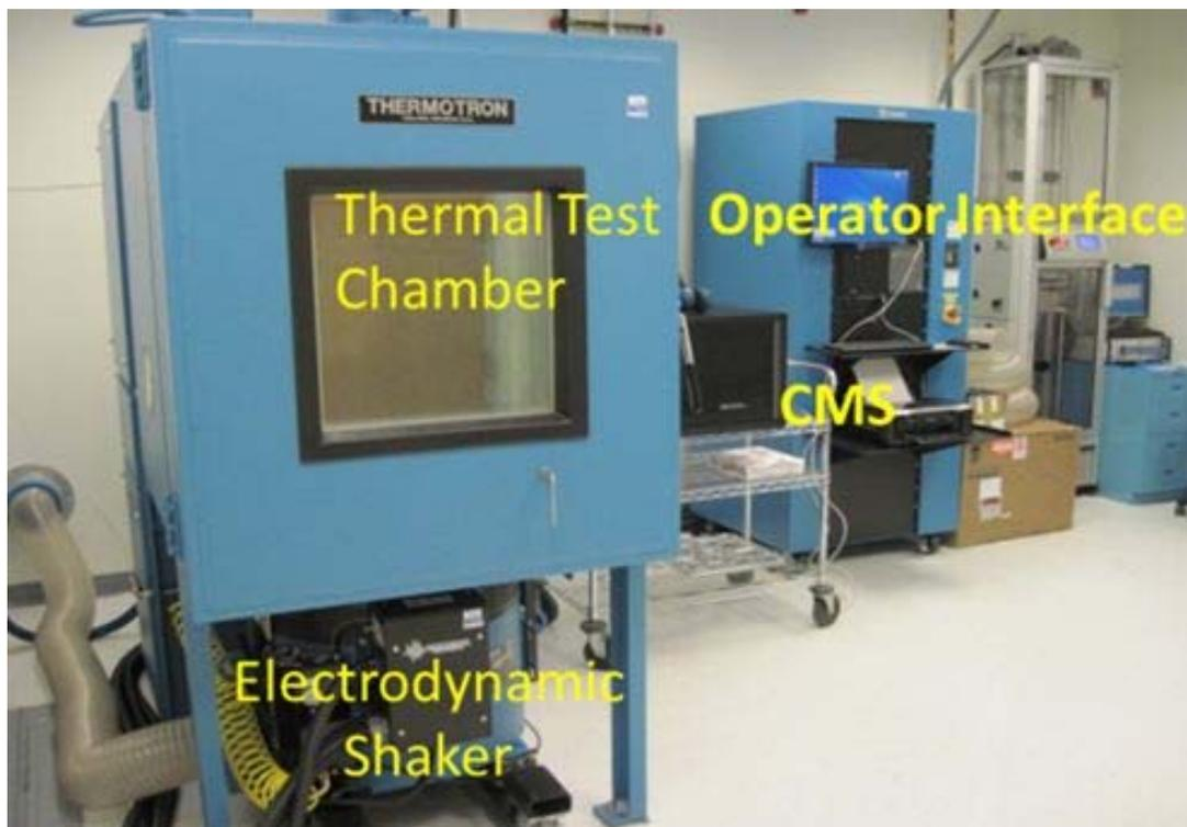
Figure 94. Thermotron DXS-2250 Vibration Tester
