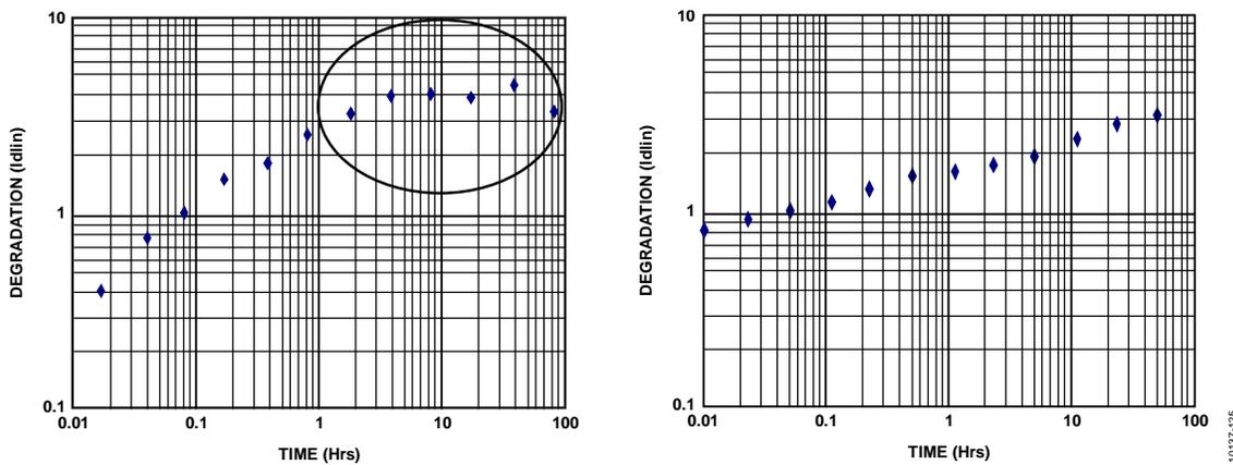
Figure 27. Effect of 1-Hour Recovery Period Post Stressing
