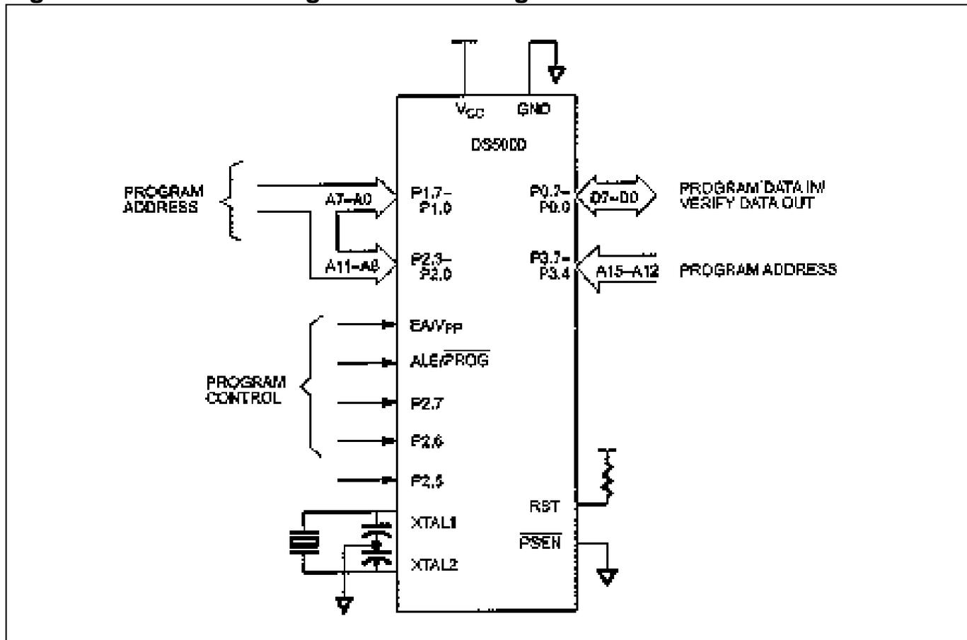
**Figure 16-4. Parallel Program Load Cycles**
