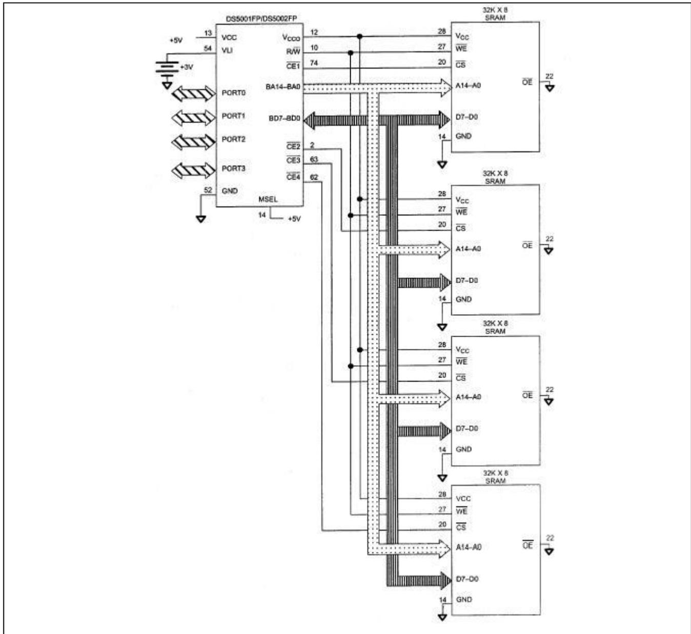
**Figure 5-5. Memory Interconnect Using the 128kB SRAM**
