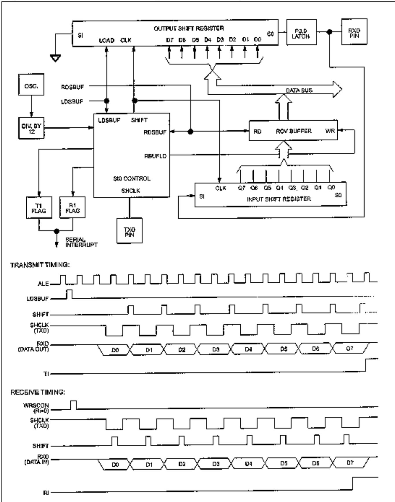
Figure 14-3. Mode2 and 3 Block Diagram
