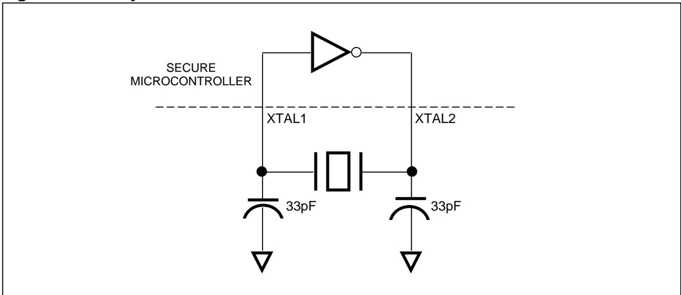
**Figure 15-2. Clock Source Input**
