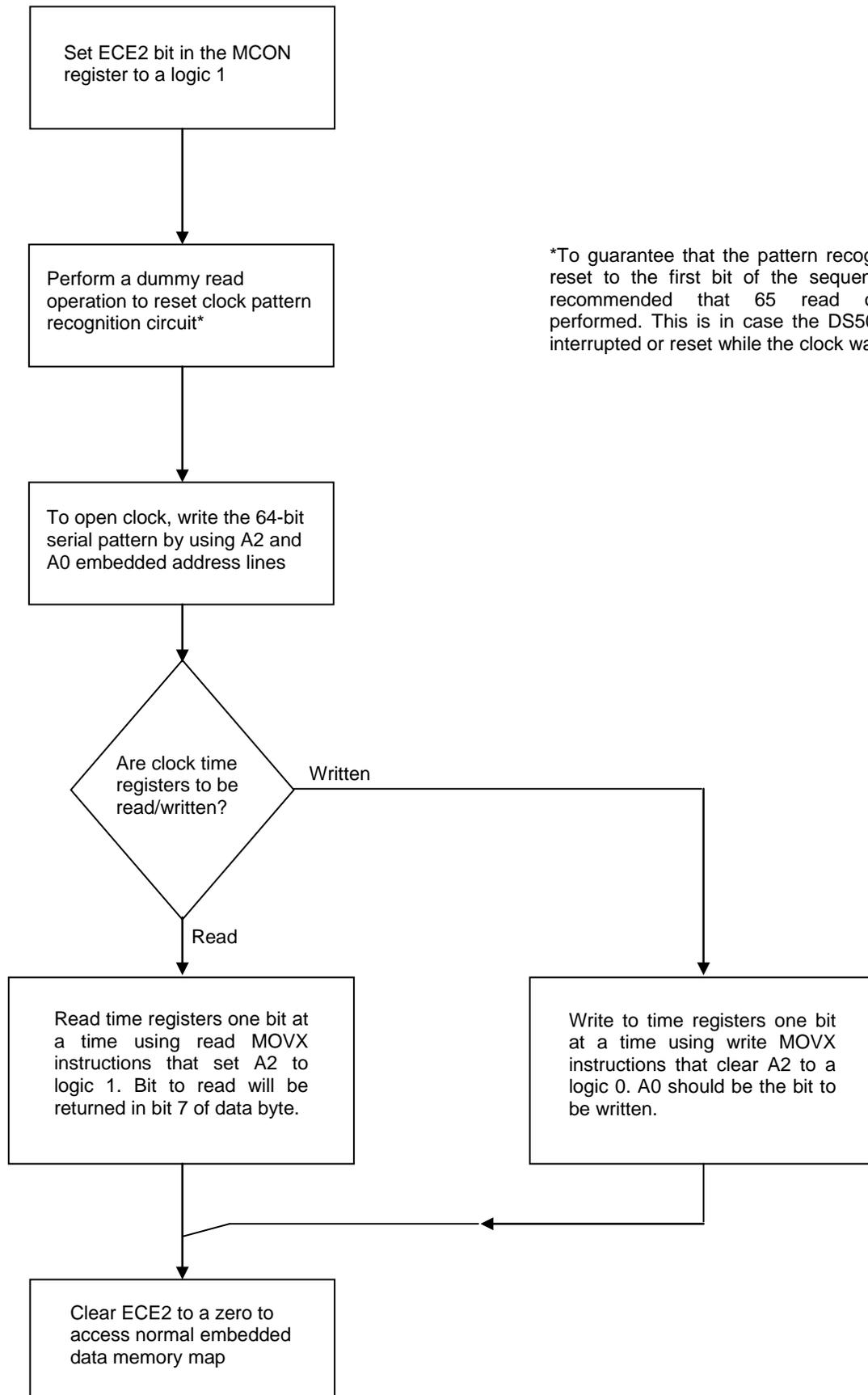
**Figure 17-4. DS5000T/DS2250T RTC Registers**
