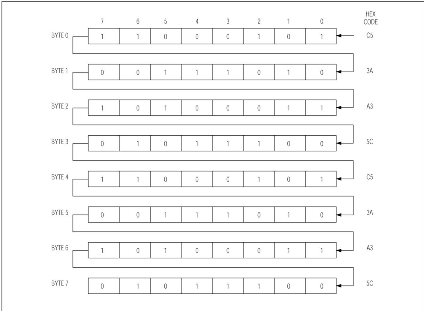
**Figure 17-3. DS5000T/DS2250T RTC Register Entry Flowchart**
