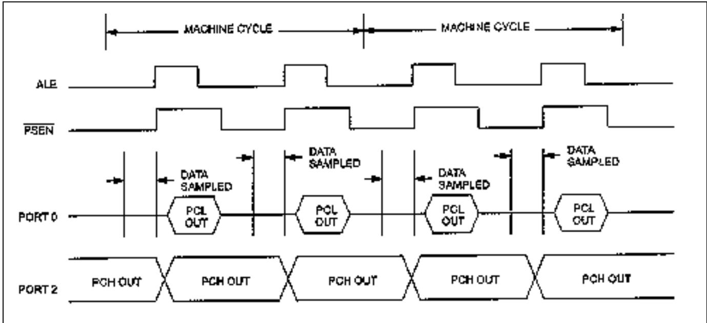
Figure 15-5. Expanded Data Memory Read
