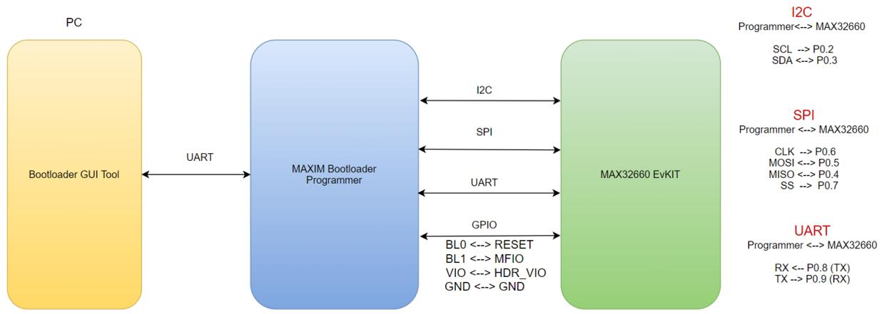
Figure 10. The overall system required pin connections.
