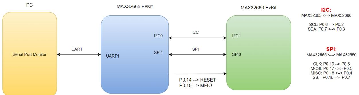
Figure 19. Bootloader host example setup block diagram
