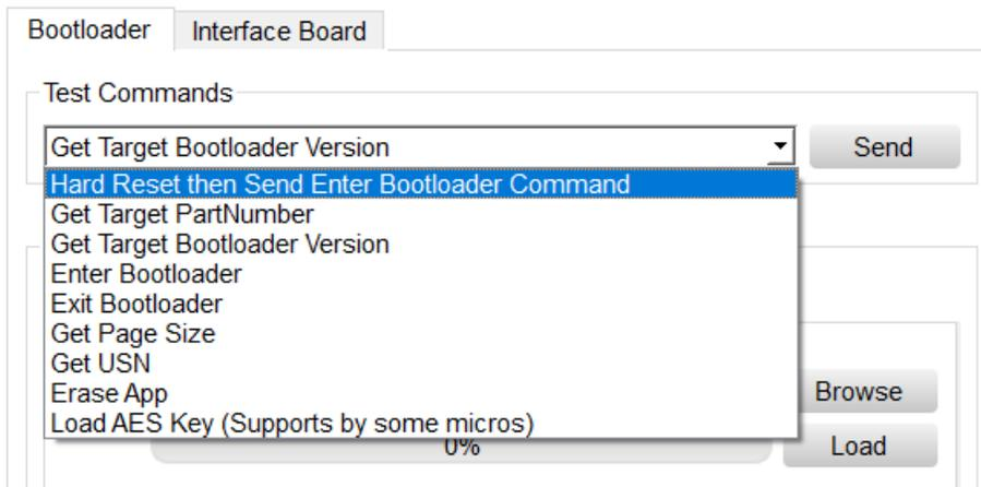
Figure 14. Bootloader test command.
