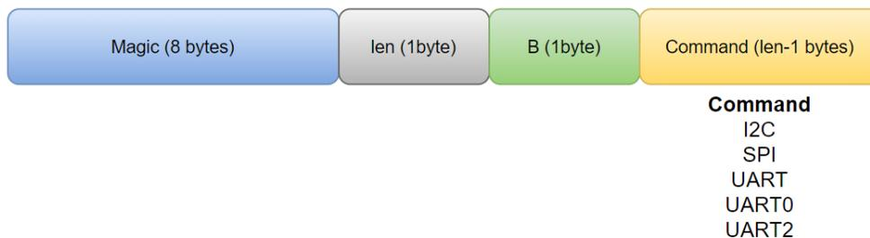
*Figure 31. Request packet (from PC to interface board).*
