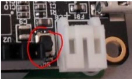
Figure 7. MAX32630FTHR host reset button.
