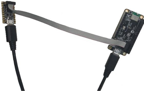
Figure 3. The MAX32630FTHR and MAX32625PICO board connection.
