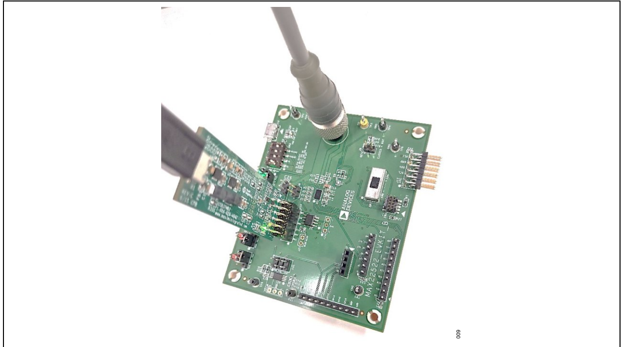
Figure 8. USB2PMB2 Connection to Program On-Board EEPROM
