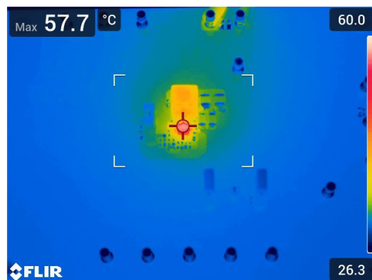
LT80603 EVALUATION BOARD CONDITIONS: 5V OUTPUT, 3.5A, f_{SW} = 400\text{kHz}
