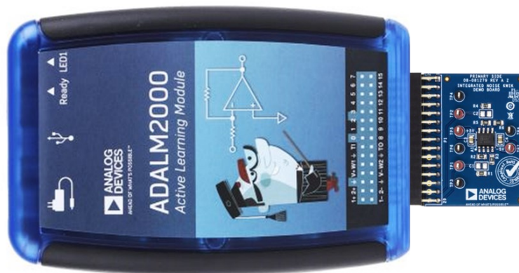
Figure 4. Connecting EVAL-KW4501Z to ADALM2000
