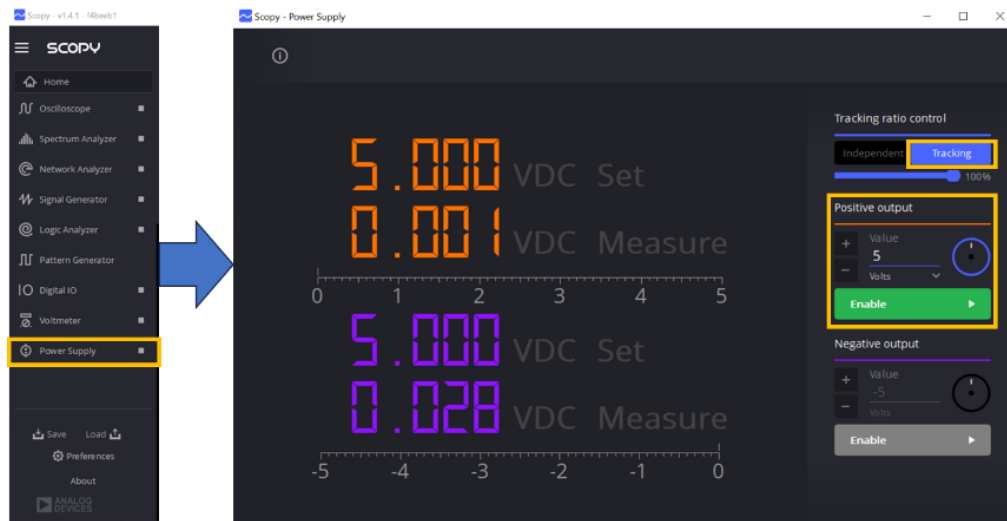
Figure 8. Setting the Power Supply
