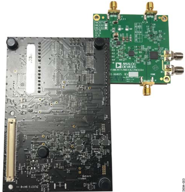
Figure 3. SDP-K1 Board Mounted to the EV1HMC8074LP6G
