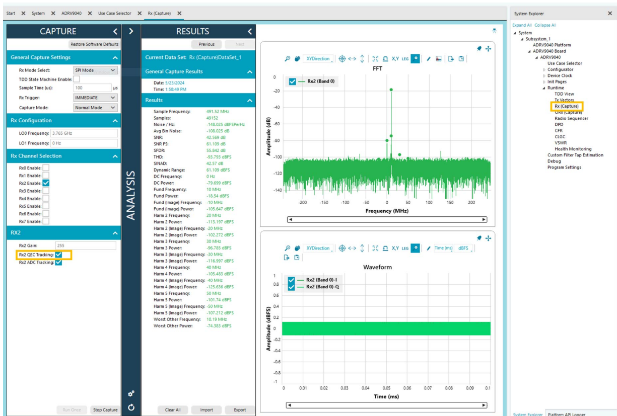
Figure 56. Rx Capture Performed after Enabling Rx QEC Tracking for Rx0
