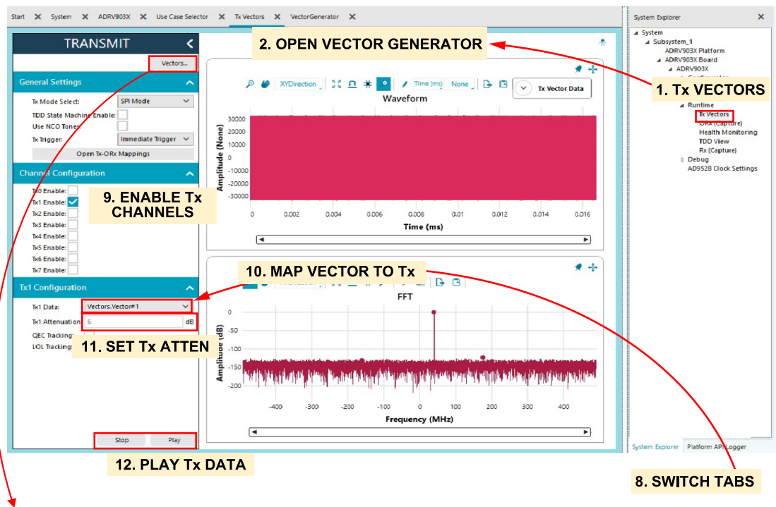
Figure 43. Tx Vectors Page is Used to Enable Tx Channels, Map Vectors to Each Enabled Tx, and Plot the Baseband Vectors
