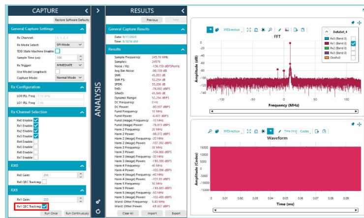
Figure 48. Rx Capture Performed after Enabling Rx QEC Tracking for Rx0
