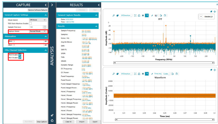
Figure 49. ORx0 and ORx1 Data Captured over JESD Link with Tx LO and 10MHz Input Tone Applied to ORx0
