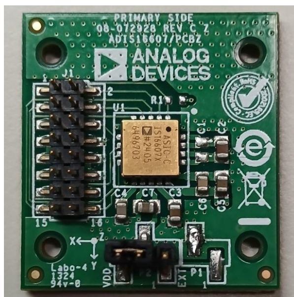
Figure 1. ADIS16607-x/PCBZ Evaluation Board Photograph
