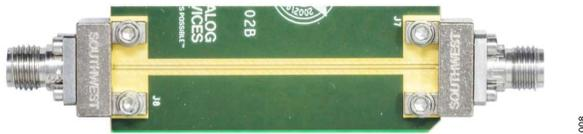
Figure 8. EVAL-ADGM1121SDZ Calibration Transmission Line Used for PCB Insertion Loss and Phase Offset Correction
