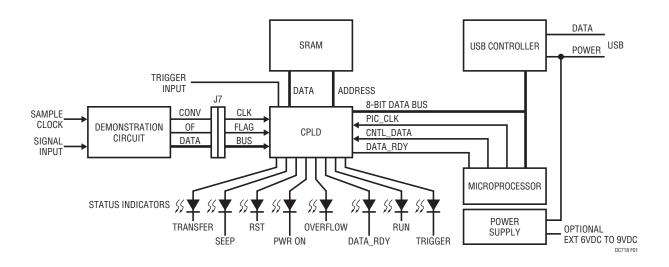
Figure 1. DC718 Block Diagram
