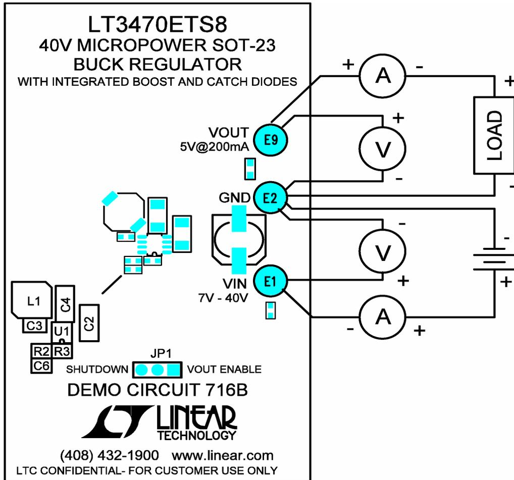
INSTALL SHUNT AT JP1: PINS 1 & 2 = VOUT ENABLE
