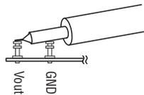
**Figure 2. Scope Probe Placement for Measuring Output Ripple**
