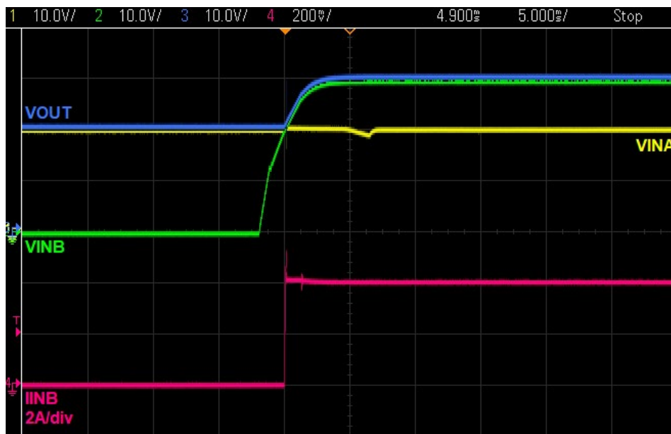
Figure 4. Diode-OR Using Figure 2. VINB Ramps to Higher Voltage than VINA. VOUT Follows VINB, which Supplies the Full Load Current
