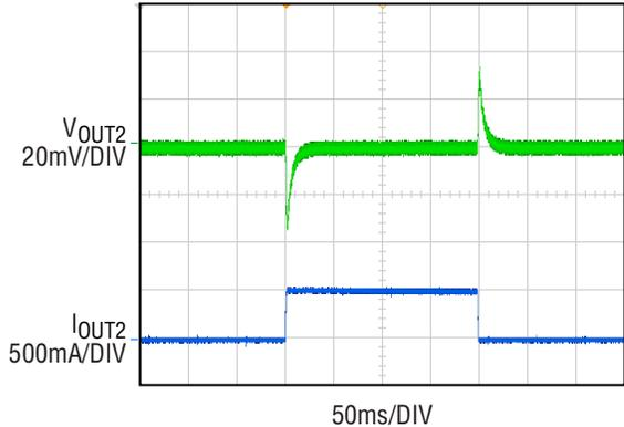
Figure 8. Load Step at  $V_{IN} = 3.3V$ ,  $V_{OUT2} = 1.8V$ ,  $f_{SW} = 2MHz$
