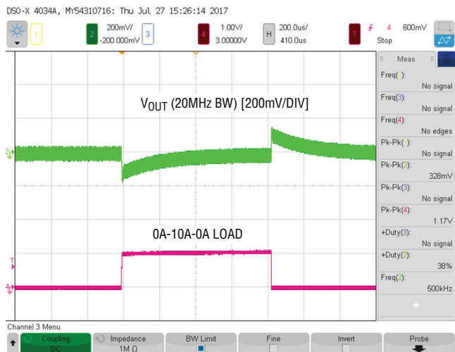
Figure 5. Load Step at V_{IN} = 48V , V_{OUT} = 12V
