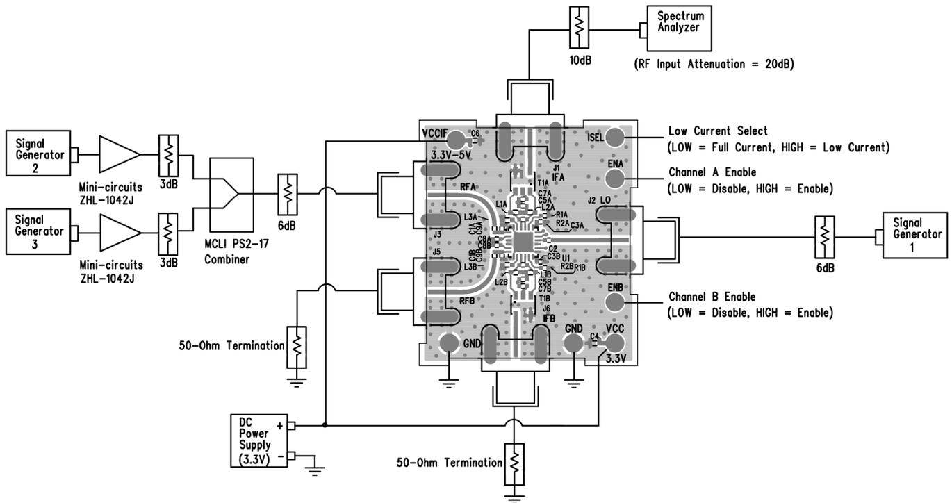
Figure 2. Proper Equipment Setup for RF Performance Measurements
