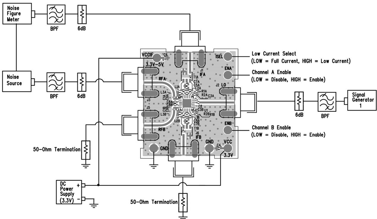
Figure 3. Proper Equipment Setup for Noise Figure Measurement
