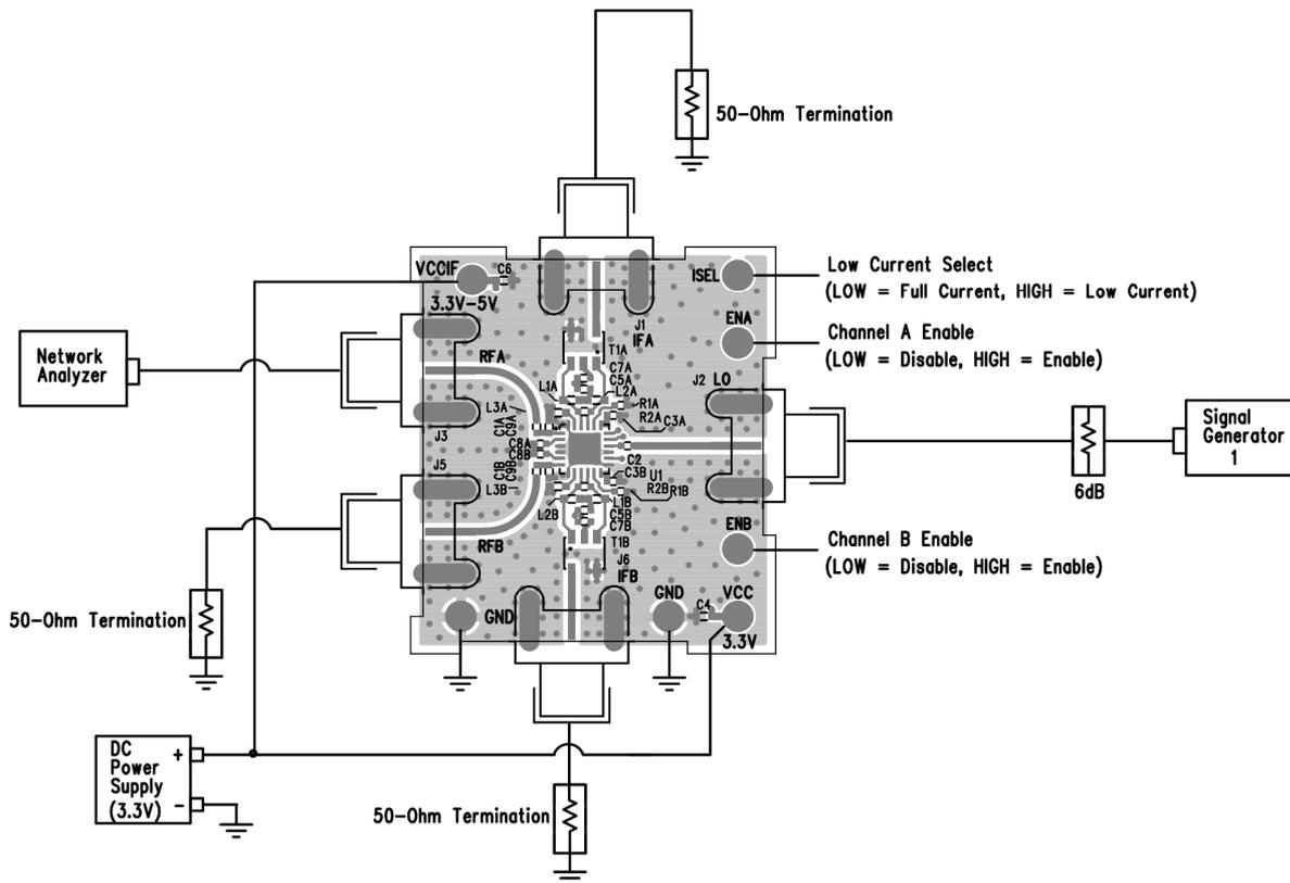
Figure 1. Proper Equipment Setup for Return Loss Measurements
